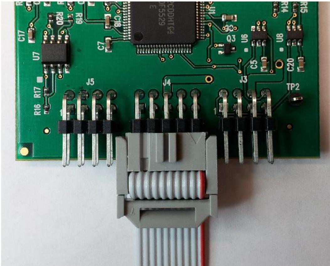
Figure 15. 10-pin Cable Connection to J4
