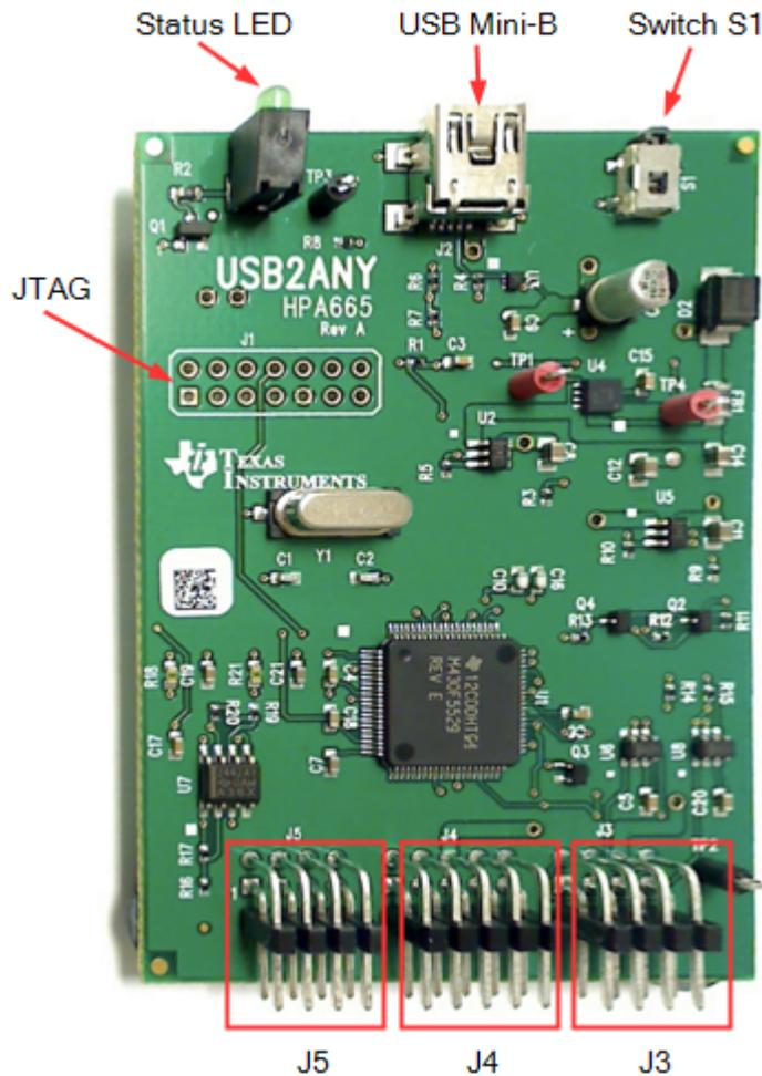
**Figure 14. USB2ANY Board Connections**
