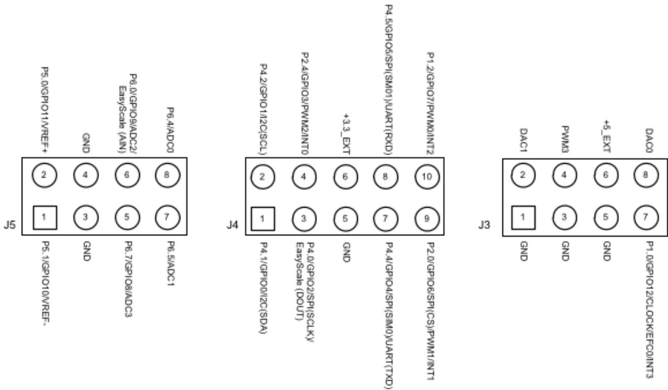
Figure 17. USB2ANY Board Connector Pinout Diagram
