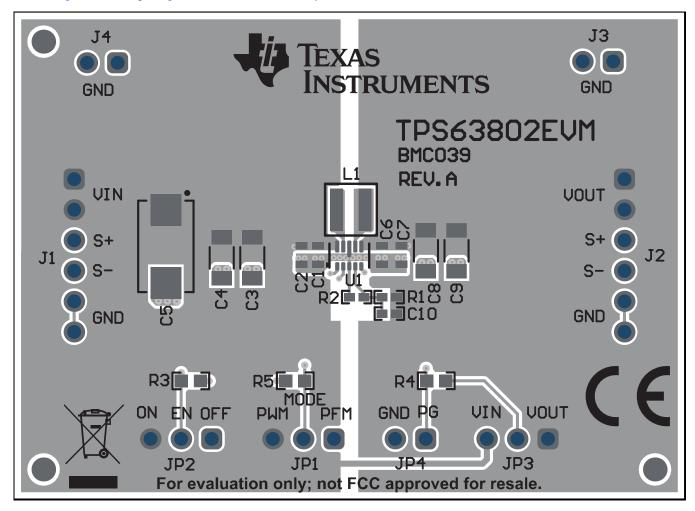
Figure 2. Assembly Layer
