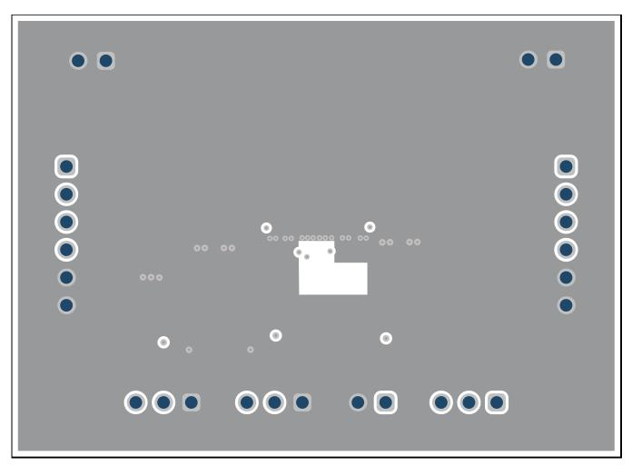
Figure 5. Bottom Layer Routing
