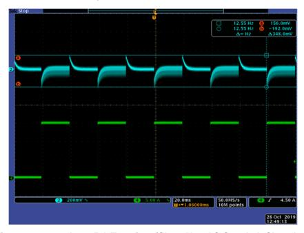
Figure 19. 300 mA to 15 A Transient (Ch2 =  $V_{OUT}$  AC Coupled; Ch4 =  $I_{OUT}$ )
