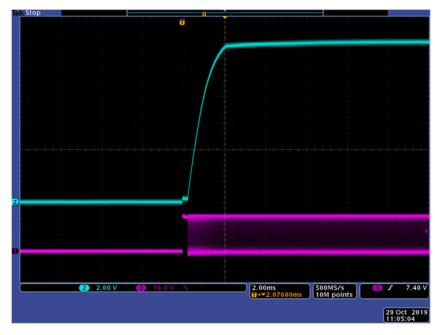
Figure 14. Full Load (15 A) Startup (Ch2 = V<sub>OUT</sub>; Ch3 = LO)
