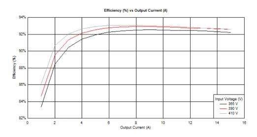
Figure 8. Efficiency vs Output Current
