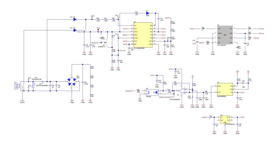
Figure 4. UCC25640EVM-020 Control Schematic
