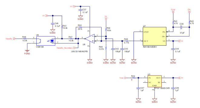
Figure 30. External Standby Circuit Current Sense Gain and Comparator
