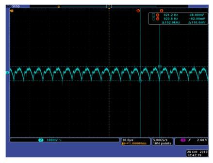
Figure 18. Full Load (15 A) Output Ripple (Ch2 =  $V_{OUT}$ )
