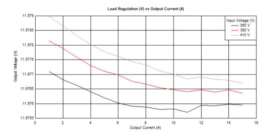
Figure 9. Load Regulation vs Output Current
