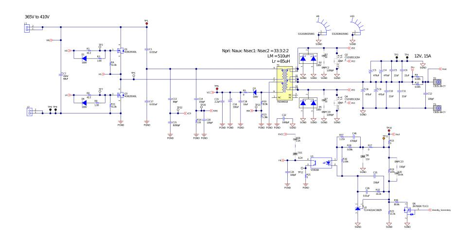
Figure 3. UCC25640EVM-020 Power Stage Schematic
