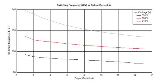
Figure 10. Switching Frequency vs Output Current
