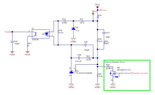
Figure 31. Output Voltage Set Point Adjustment
