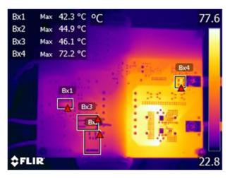
Figure 16. Thermal Image Bottom
