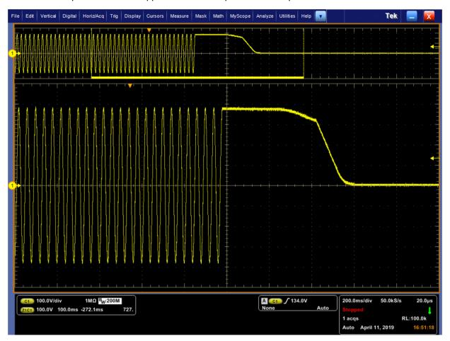
Figure 24. X-Cap Discharge (Ch1 = Voltage across X-Cap, C40 and C41)
