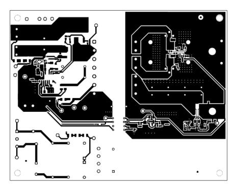
Figure 28. UCC25640EVM-020 Bottom Copper Assembly Drawing (Top view)
