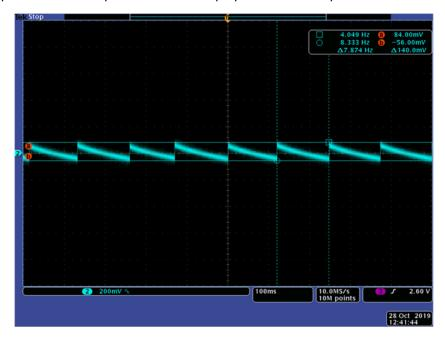
Figure 17. No Load (0 A) Output Ripple (Ch2 =  $V_{OUT}$ )
