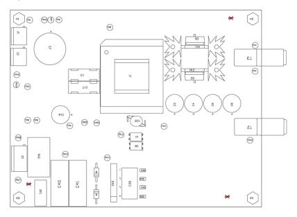
Figure 25. UCC25640EVM-020 Top Layer Assembly Drawing (Top view)
