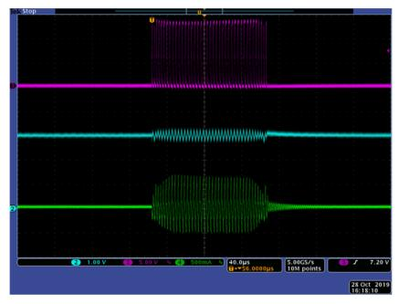
Figure 22. Steady State Waveforms at No Load (Ch2 = VCR; Ch3 = LO; Ch4 = IResonant)
