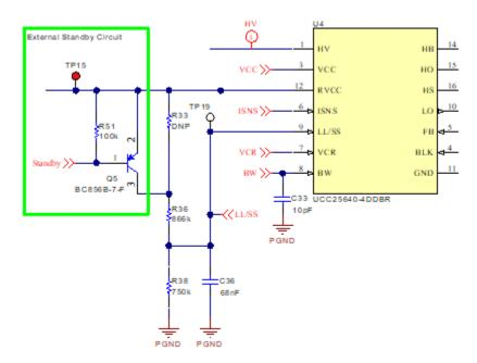
Figure 32. Burst Mode Threshold Adjustment
