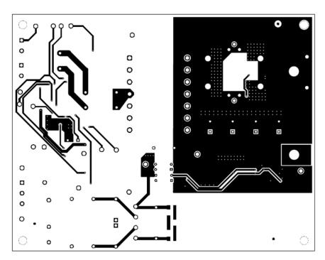
Figure 27. UCC25640EVM-020 Top Copper Assembly Drawing (Top view)
