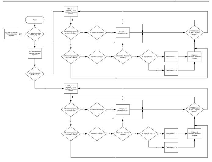
Figure 5-1. BTP Algorithm Flow
