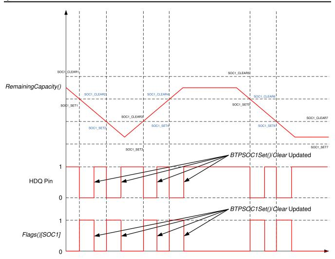
Figure 5-2. BTP Configuration with Multiple Thresholds
