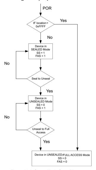
Figure 16-1. Gauge Mode State Diagram
