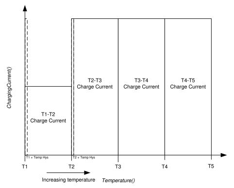
Figure 7-3. Temperature Hysteresis for Charging Current
