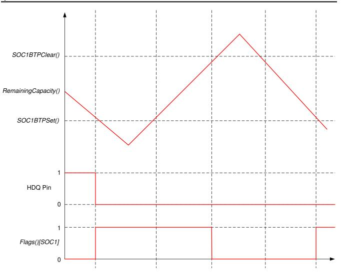
Figure 5-4. BTP Configuration with Separate Thresholds
