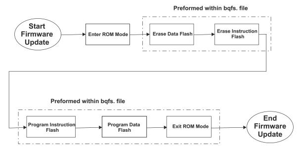
Figure 18-2. Basic Firmware Programming Flow
