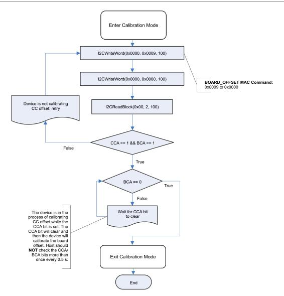
Figure 17-2. Board Offset Flow
