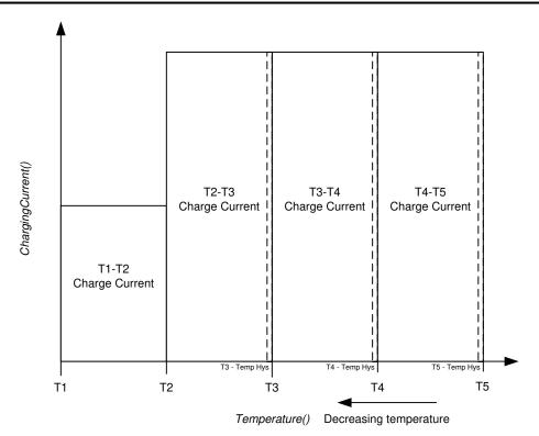
Figure 7-4. Temperature Hysteresis for Charging Voltage
