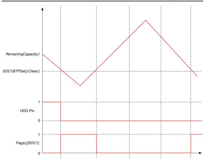
Figure 5-3. BTP Configuration with Shared Thresholds
