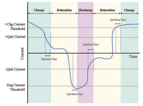
Figure 6-1. Example of Algorithm Operation Mode Changes With Varying DataRAM.EffectiveCurrent()
