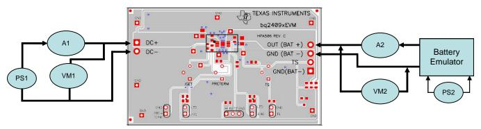
Figure 1. Original Test Setup
