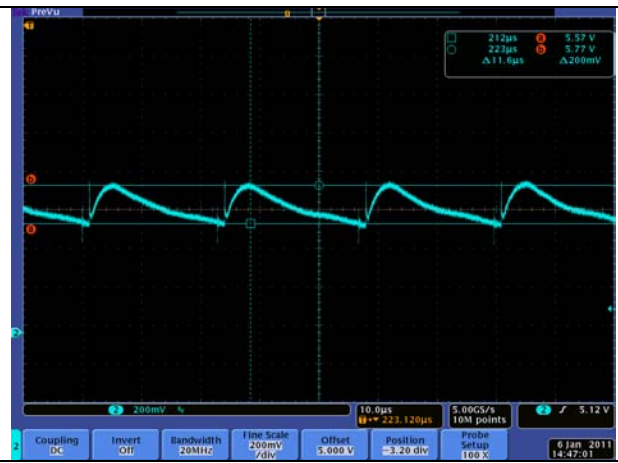
230Vin half load Ripple
