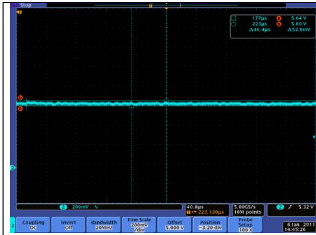
115Vin no load Ripple
