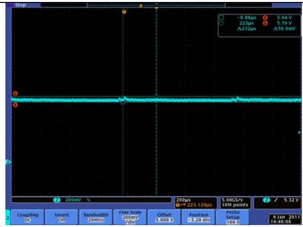
230Vin no load Ripple
