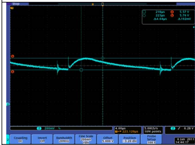
115Vin half load Ripple
