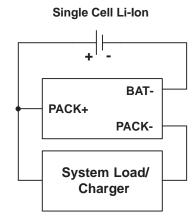
Figure 8. bq27x10EVM Circuit Module Connection to Cells and System Load/Charger
