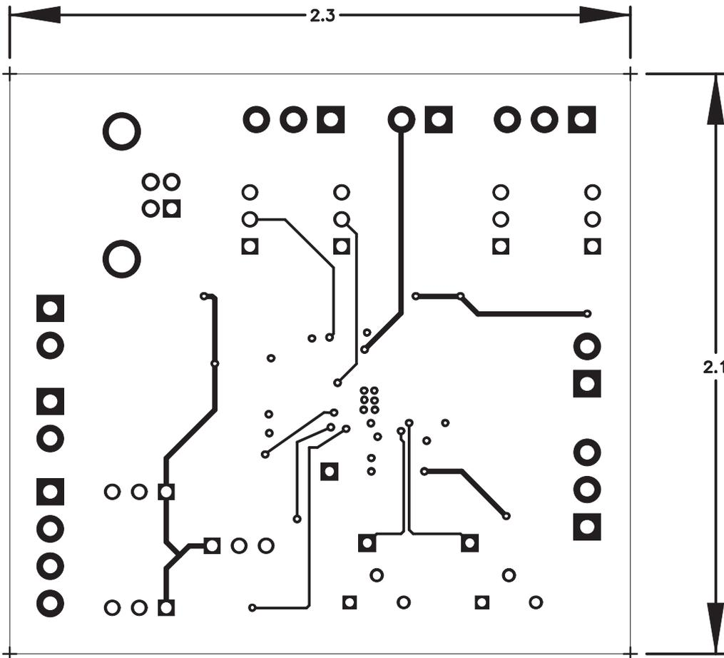
Figure 5. Board Layout – Second Etch Layer
