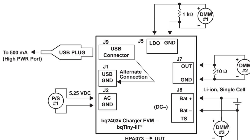
**Figure 1. Test Diagram**
