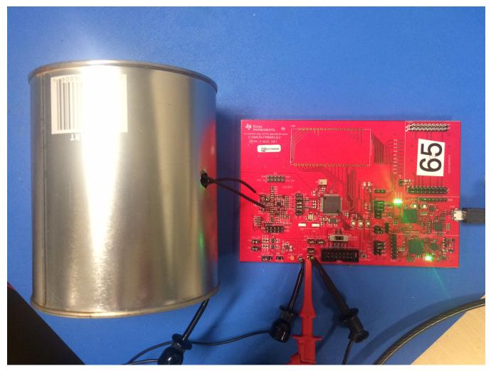
Figure 2. EVM430-FR6043 connected to gas flow meter embedded in grounded can
