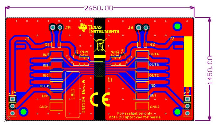
Figure 7. ISO7041DBQ PCB Layout
