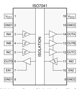
Figure 1. ISO7041 Low-Power Digital Isolator Pin Configurations
