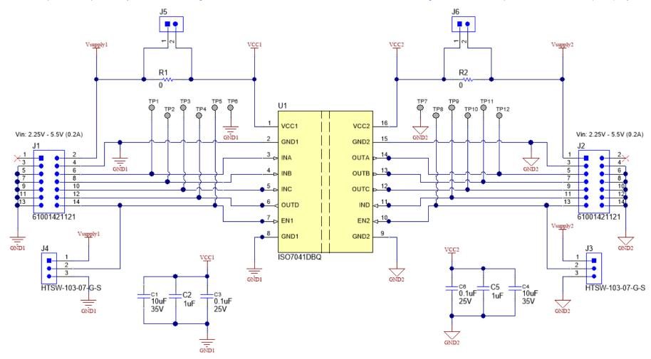
Figure 6. ISO7041DBQ EVM Schematic
