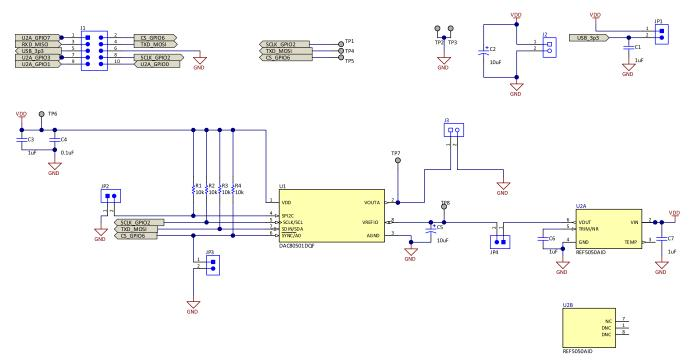
Figure 11. DAC80501EVM Board Schematic
