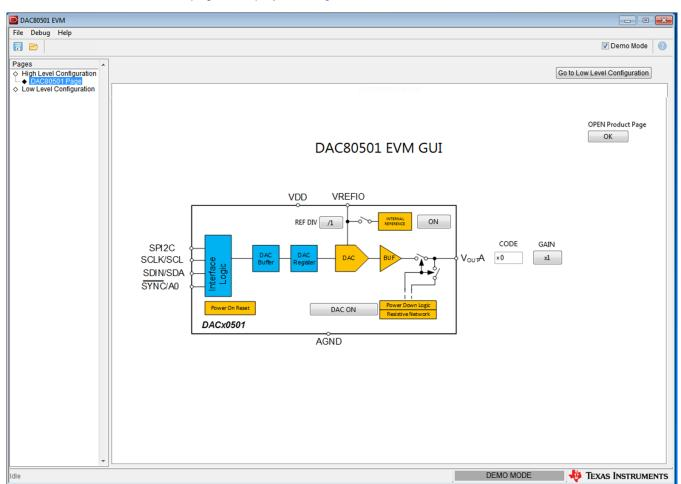
Figure 10. High Level Configuration Page
