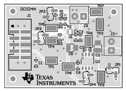
Figure 12. DAC80501EVM PCB Components Layout
