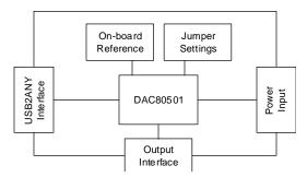
Figure 4. DAC80501EVM Hardware Block Diagram
