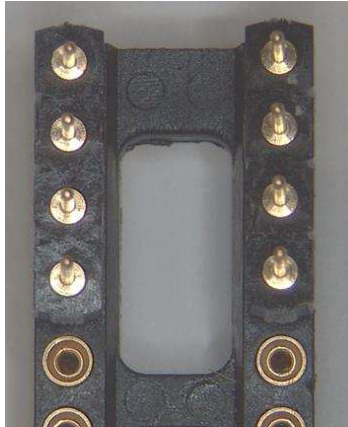
Figure 5. Terminal strip (TS-132-G-AA) inserted into spare DIP socket
