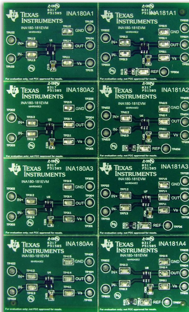
This user's guide describes the characteristics, operation, and use of the INA180-181 evaluation module (EVM). This EVM is designed to evaluate the performance of the [INA180A1](#), [INA180A2](#), [INA180A3](#), [INA180A4](#), [INA181A1](#), [INA181A2](#), [INA181A3](#), [INA181A4](#) voltage output current-shunt monitors in a variety of configurations. This document includes a schematic, reference printed-circuit board (PCB) layouts, and a complete bill of materials.
