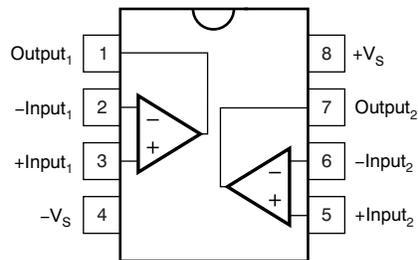
**Figure 1. MSOP-8 Package Pinout, Top View**
