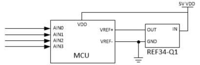
Figure 11. External ADC Referencing With REF34-Q1
