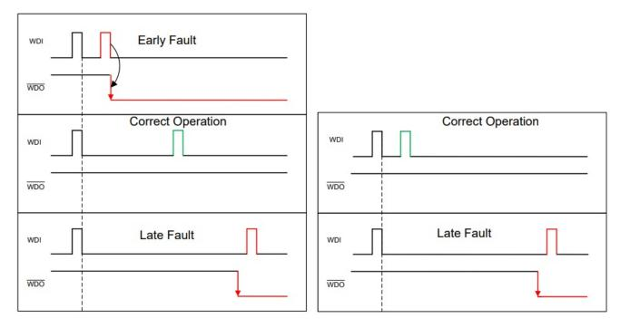
Figure 5. Window Watchdog (Left) Vs. Standard Watchdog (Right)
