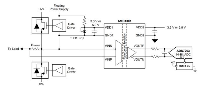
Figure 12. High Voltage Current Monitoring Application Design
