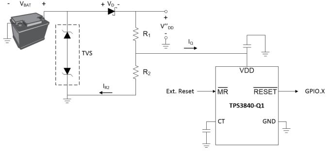
Figure 9. Illustrating TPS3840-Q1 Implementation For Wide-V<sub>IN</sub> Designs
