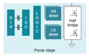
Figure 16. Power Stage Entities And Functional Blocks
