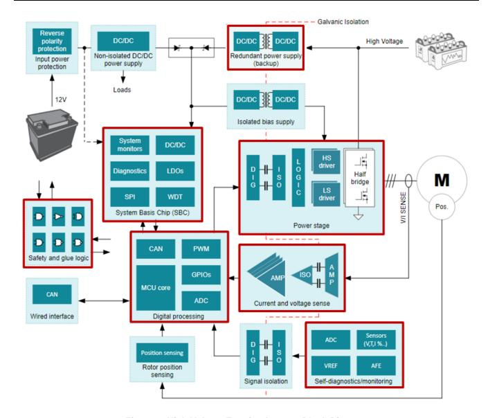
Figure 2. High Voltage Traction Inverter Block Diagram
