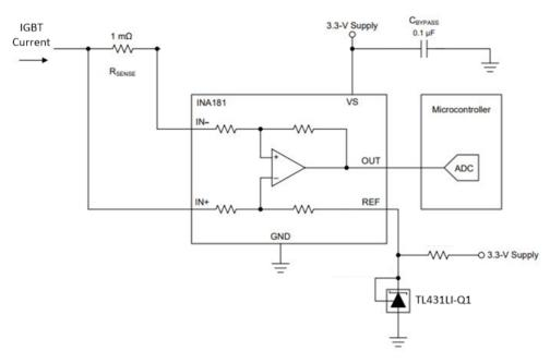
Figure 15. Current Sensing With INA181-Q1 and TL431LI-Q1
