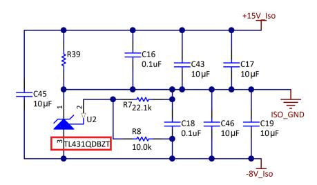
Figure 17. Negative Voltage Supply Generation With TL431LI-Q1 in TIDA-020015
