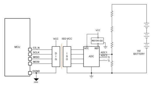
Figure 13. High-Side Voltage Sense Design Approach
