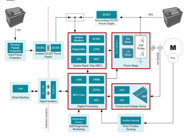
Figure 1. Starter Generation Unit Block Diagram
