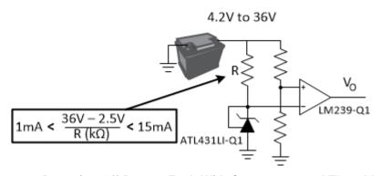
Figure 8. Detecting Off-Battery Fault With Comparator and TL431LI-Q1
