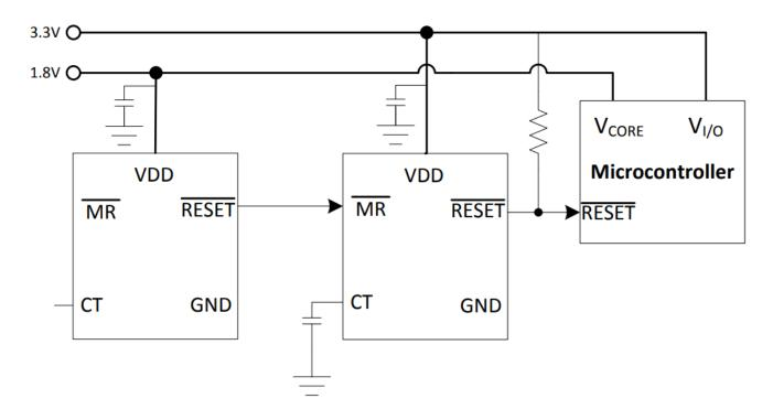
Figure 4. Micrcontroller Supply Monitoring With Voltage Supervisor(s)
