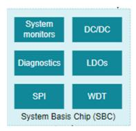
Figure 3. System Basis Chip Entities And Functional Blocks
