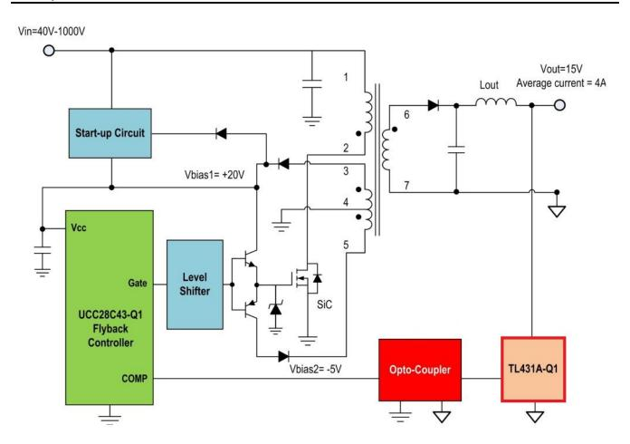
Figure 19. Isolation Compensation with TL431A-Q1 in TIDA-01505
