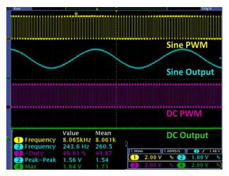
Figure 3. C2 = 220 pF, 1.64 VDC, 50% PWM
