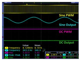
Figure 4. C2 = 420 pF, 3.32 VDC, 100% PWM
