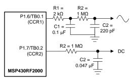
Figure 2. Output Filter Diagram
