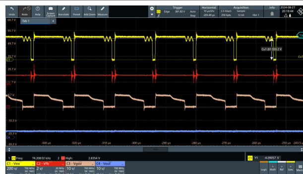
图 3-23. V_{in} = 230Vac , V_{out} = 5V
