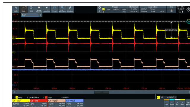
图 3-9. V_{in} = 90\text{Vac} , V_{out} = 20\text{V}
