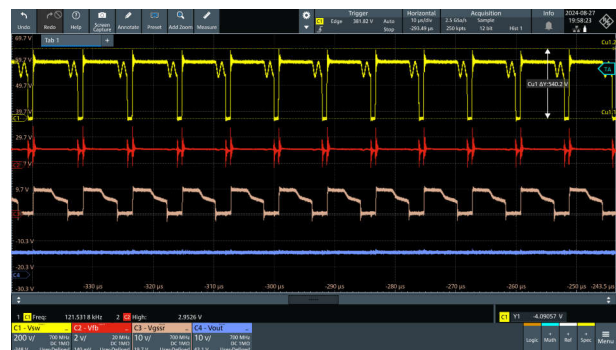
图 3-20. V_{in} = 264V_{ac} , V_{out} = 9V
