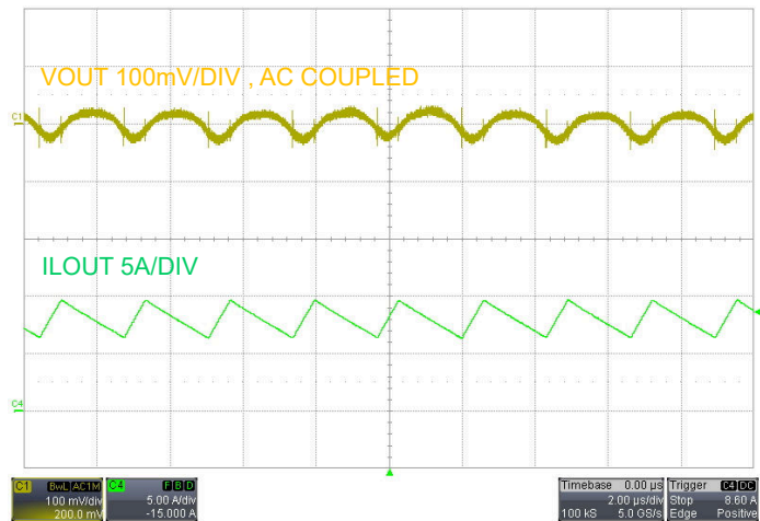
图 3-5. 输出纹波, V_{\text{SUPPLY}} = 48\text{V} , I_{\text{LOAD}} = 8\text{A}
