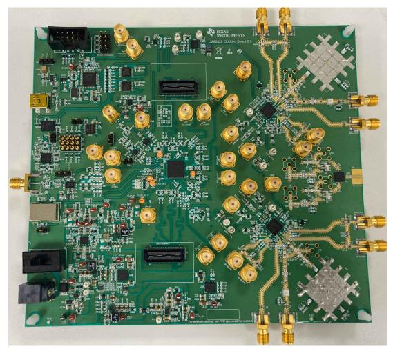
图 2-1. Multichannel Clocking Board
