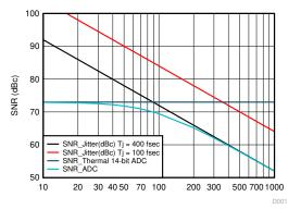
图 1-5. SNR Performance vs Input Frequency
