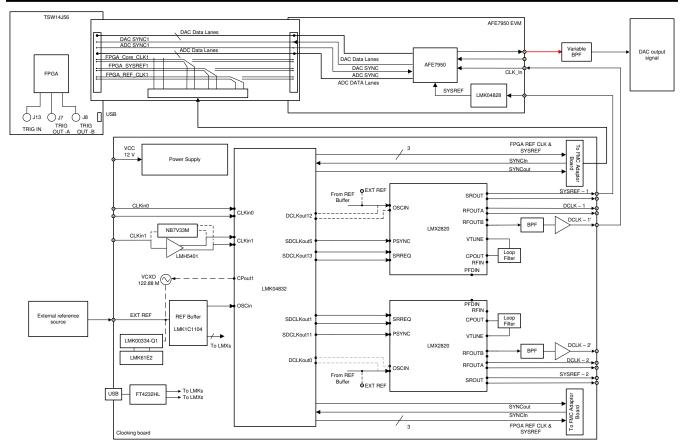
图 2-9. Test Setup for AFE7950 Receiver SNR Measurement
