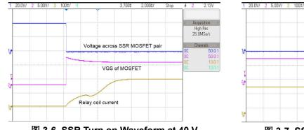
图 3-6. SSR Turn on Waveform at 40 V
