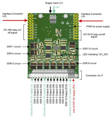
图 3-1. Input and Output Connectors in the Reference Design Board
