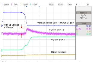
图 3-15. Test Waveforms Showing Least Cross-Coupling During SSR Turn On
