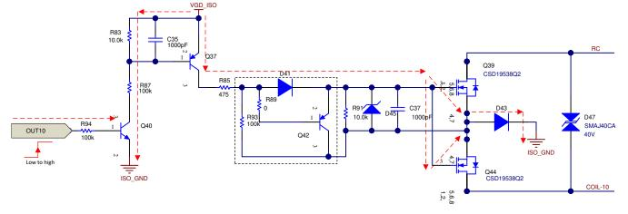
图 2-9. Gate Driver Circuit for the SSR MOSFETs and the Turn on Gate Current Path
