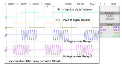
图 3-16. Test Waveforms at 24-VAC Supply - Independent Operation of SSR
