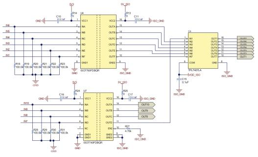
图 2-11. Digital Isolator Interface for Ten Channel SSR
