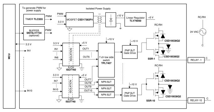
图 2-2. TIDA-010085 Reference Design Block Diagram
