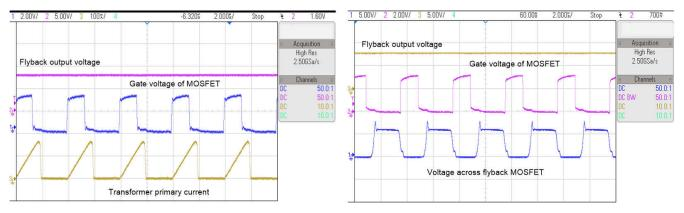
图 3-4. Flyback Circuit Voltage and Current Waveforms - All SSR On
