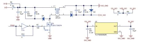
图 2-12. Open-Loop Flyback Power Supply
