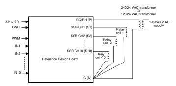
图 3-2. Interfacing External Control Signals, Relay coils and Transformer to the Board
