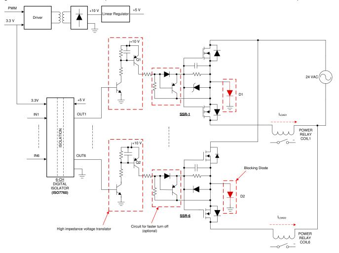
图 2-6. Circuit Topology to Drive Multiple SSR With Single Isolating Element
