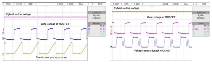
图 3-5. Flyback Circuit Voltage and Current Waveforms - All SSR Off
