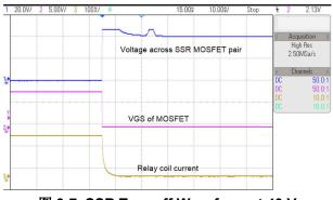
图 3-7. SSR Turn off Waveform at 40 V
