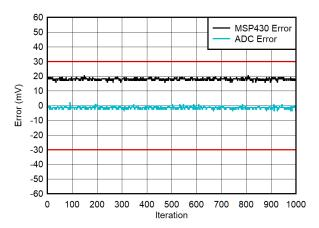
图 3-13. Noise Floor (±2-A Range, -2 A, 1-V Input)
