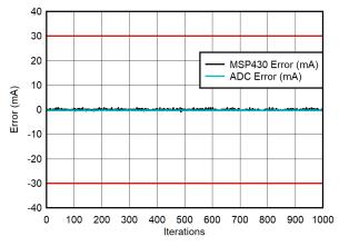
图 3-12. Noise Floor (0.25- to 1-A Range, 0 A, 5-V Input)
