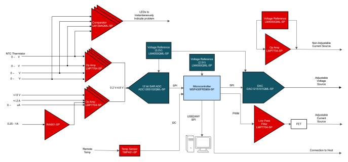
图 2-1. System Block Diagram (External ADC Configuration)
