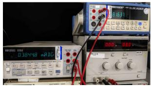
图 3-18. Constant Current Output Test Setup (8 V Applied)
