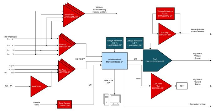
图 2-2. System Block Diagram (Internal ADC Configuration)
