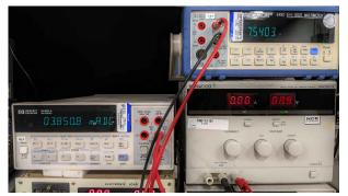
图 3-17. Constant Current Output Test Setup (7.5 V Applied)
