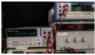
图 3-19. Constant Current Output Test Setup (9 V Applied)
