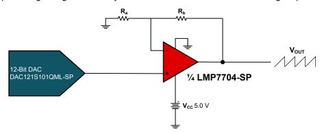
图 2-8. Adjustable Voltage Source
