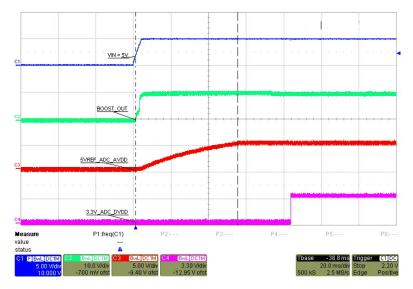
图 2-12. ADC128S102-SP Start-up Power Sequence
