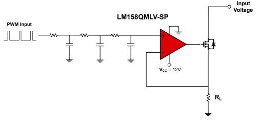
图 2-10. Adjustable Current Source Circuit
