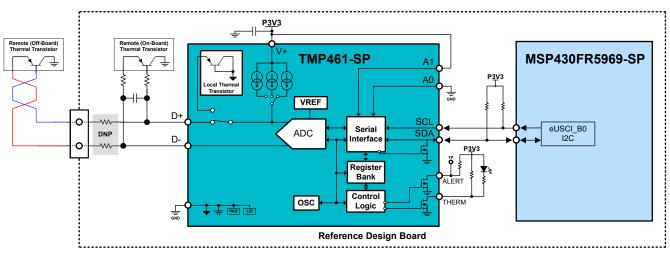
图 2-6. TMP461-SP - Local and Remote Temperature Sensing
