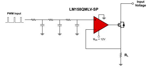
图 2-9. Fixed Output Current Source
