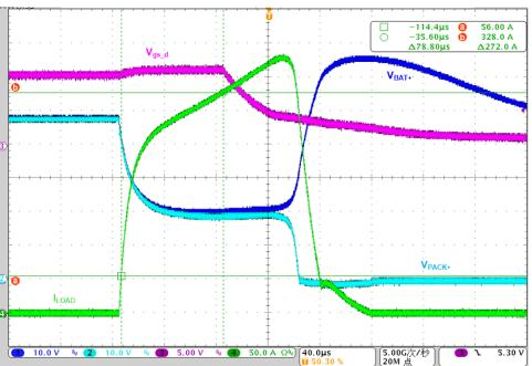
图 19. Short-Circuit Discharge Protection
