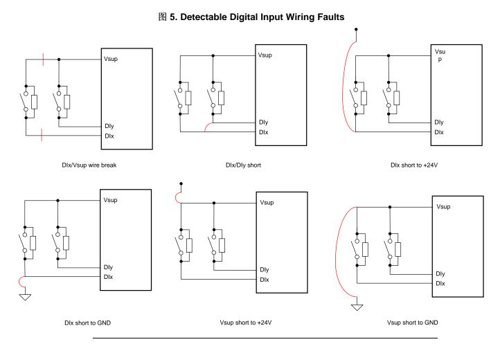
注: A resistor of 100 k $\Omega$  bypassing the switching element of the external sensor is required to detect all shown wiring faults including wire-break detection.
