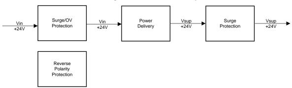
Powering the external sensors straight from a 24-V DC field power supply source is possible, but wire diagnostics is limited in this case as the module does not control the power for the external sensors.
