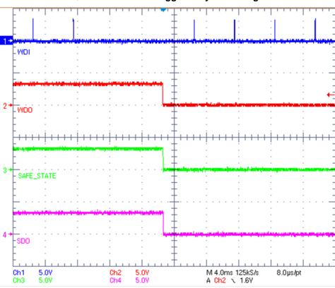
图 10. Safe-State Triggered by Watchdog
