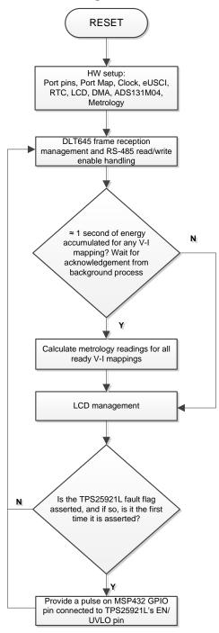
The initialization routines involve the setup of the MSP432 general purpose input/output (GPIO) port pins and associated port map controller; MSP432 clock system; MSP432 USCI\_A0 for UART functionality; MSP432 RTC module for clock functionality; MSP432 LCD; MSP432 DMA; ADS131M04 registers; and MSP432 metrology variables.
