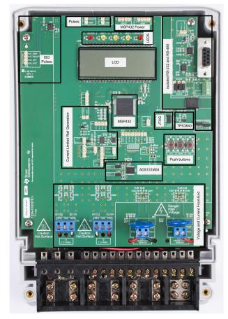
The design has support for two-voltage and one-voltage configurations. The hardware connections depend on which of these two configurations is selected.
