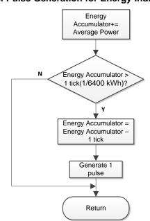
图 16. Pulse Generation for Energy Indication
