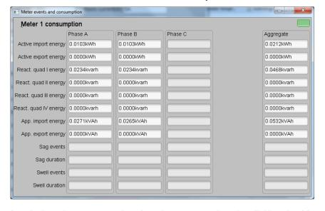
图 29. Meter Events and Consumption Window
