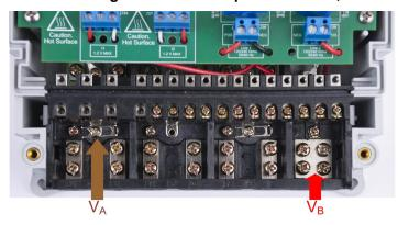
$\boxtimes$  22 shows the connections from the front view.  $V_A$  and  $V_B$  correspond to line A and line B.  $I_A$ + and  $I_A$ correspond to the current inputs for line A while  $I_B$ +, and  $I_B$ - correspond to the current inputs for line B.
