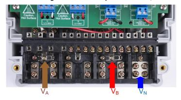
$\boxtimes$  20 shows the connections from the front view.  $V_A$  and  $V_B$ , correspond to the lines for phases A and B.  $V_N$  corresponds to the neutral voltage from the test AC source.  $I_A$ + and  $I_A$ - correspond to the current inputs for phase A while  $I_B$ +, and  $I_B$ - correspond to the current inputs for phase B.
