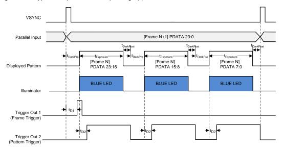
图 7. External Pattern Streaming Timing Sequence (24-bit Monochrome)
