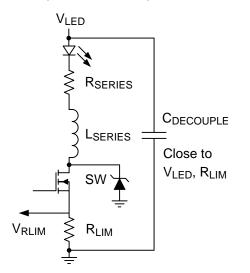
图 15. Parasitic Inductance (L<sub>Series</sub>) and Resistance (R<sub>series</sub>) in Series with LED
