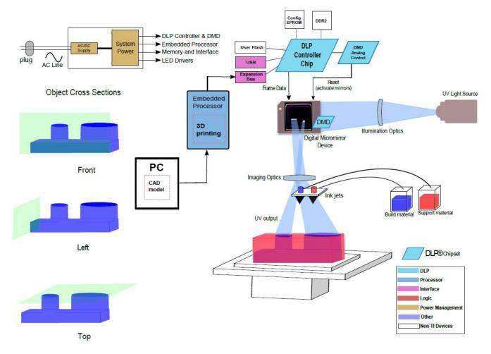
图 1 shows a typical block diagram of a 3D printing system that uses the stereolithography technique.
