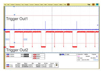
图 8. Scope plots of Trigger Out1 and Trigger Out2 (24-bit Monochrome)
