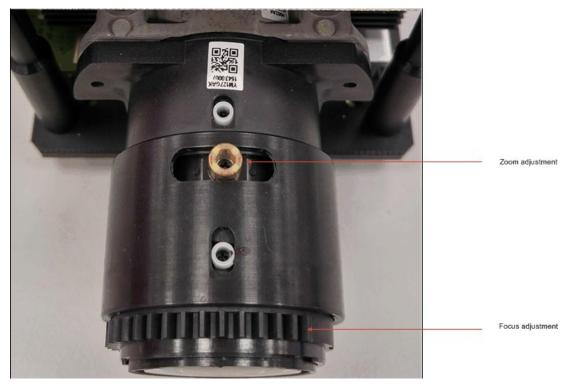
图 6. Optical Module With Focus and Zoom Adjustment
