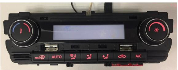
图 30. LED Dimming With 45% Duty Cycle
