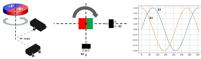
图 17. Measurement Principle of Rotating Magnetic Field
