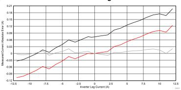
图 34. Absolute Error in Inverter Leg Current Measurement
