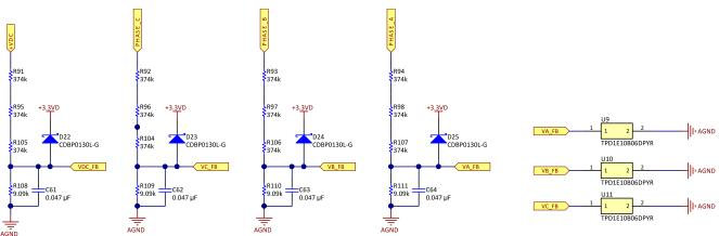
In 图 13, PHASE\_A, PHASE\_B, and PHASE\_C are the phase voltages. These voltages are properly scaled and fed to the MCU through VA\_FB, VB\_FB, and VC\_FB. The maximum phase voltage feedback measurable by the MCU can be calculated as 公式 16 shows, considering the maximum voltage for the ADC input is 3.3 V.
