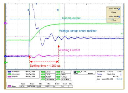
$\boxtimes$  30 and  $\boxtimes$  31 show the step response with winding current at 12 A winding current. The settling time of current sense amplifier output is 1.34 µs. Faster settling time and rail to rail output capability helps to minimize the current sense distortion especially with 2-shunt at lower phase duty cycles.
