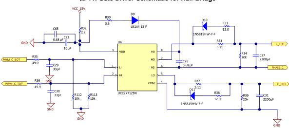
图 11. Gate Driver Schematic for Half Bridge
