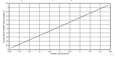
图 32. Inverter Leg Current vs Output Voltage Transfer Function Op Amp
