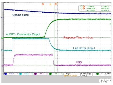
The response time of the overcurrent detection is less than 1.0  $\mu$ s in hardware protection, which is fast enough to protect an IGBT (IGBTs typically have more than a 5- $\mu$ s short-circuit capability). The lowest propagation delay of gate driver and line driver enables the fast turnoff of the IGBTs during an overcurrent event.
