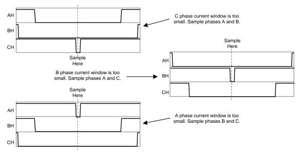
图 2. Using Three-Shunt Current Sampling Technique
