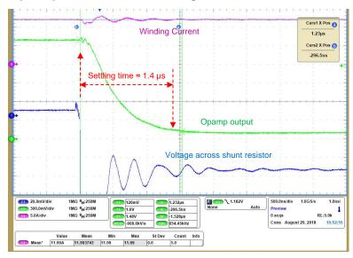
图 30. Step Response of Current Sensing Circuit With 12-A Positive Current
