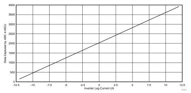
DC accuracy of the current sense amplifier TLV9064 is done with 5-m $\Omega$  sense resistor at a gain of 25.125 V/V and at 25°C ambient temperature. The full-scale DC bus current range is –13.2 A to +13.2 A. The inverter leg current is measured with a precision 6½ digit multimeter connected in series to the inverter leg shunt and the output voltage of the current sense amplifier TLV9064 is measured with another precision 6½ digit multimeter.
