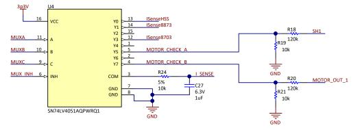
图 6. Analog Multiplexer Schematic
