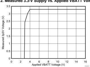
图 12. Measured 3.3-V Supply vs. Applied VBATT Voltage
