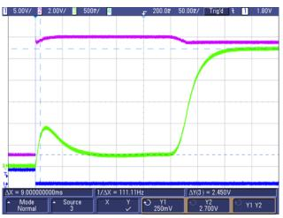
图 25. DRV8873-Q1 Motor Driving Headrest Lift Showing Motor Stall
