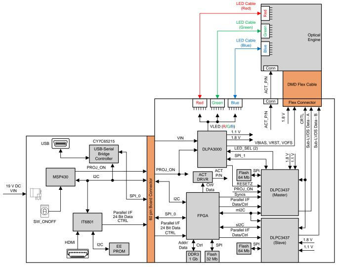
图 1. DLP LightCrafter Display EVM Block Diagram
