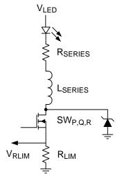
图 8. Parasitic Inductance ( $L_{series}$ ) and Resistance ( $R_{series}$ ) in Series With LED
