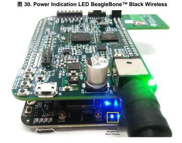
• The Blue power LED on the MIC board indicates the power on the board as 8 31 shows.
