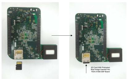
Couple the BeagleBone Black Wireless (BBB-W) and the DSP board by placing the DSP board on top of the BBB-W. Ensure the orientation of the boards prior to combining are correct as shown in 图 25. The DC Jack of BBB-W and DSP board should be aligned vertically after proper mating as shown in 图 26
