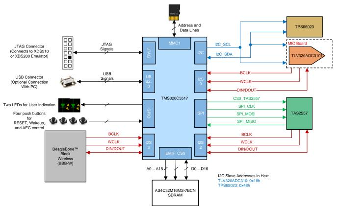
图 10. Externals Interfaces With C5517 DSP
