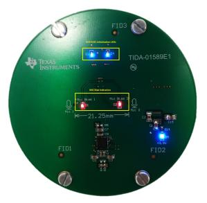
图 33. MIC BIAS and ADC3101 Initialization Indication LEDs on MIC Board
