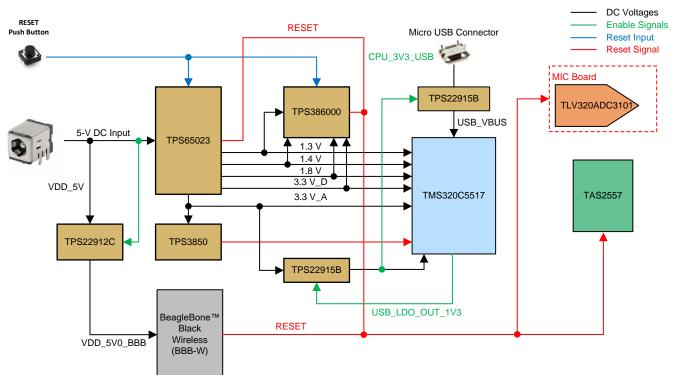
图 9. Reset and Power Sequencing
