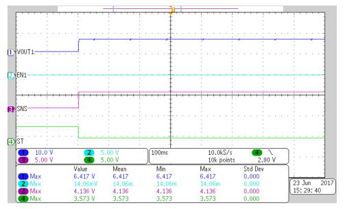
图 5. Open-Load With Switch-Disabled Test Results
