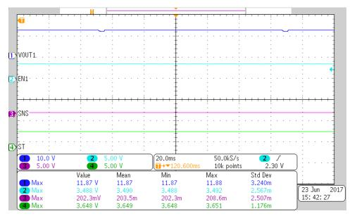
图 4. Open-Load With Switch-Enabled Test Results
