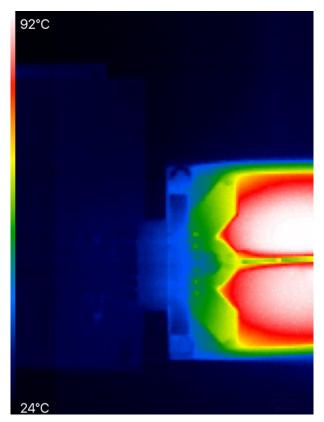
图 7. TPS1HA08-Q1 Thermal Performance Test Results
