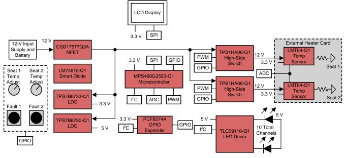
图 1. TIDA-01184 Functional Block Diagram
