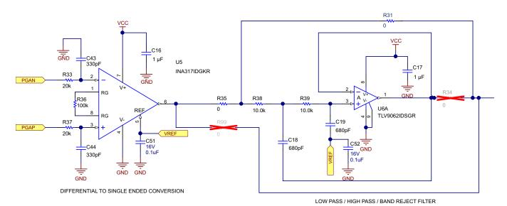
图 15. 50, 60 Hz Notch Filter Schematics for the Filter Implementation
