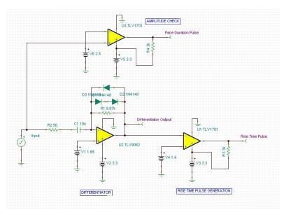
图 28. TINA-TI™ Simulation Schematic of the Signal Measurement Section Till Pulse Generation
