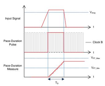
图 6. Pace Duration Pulse Generation and Measurement
