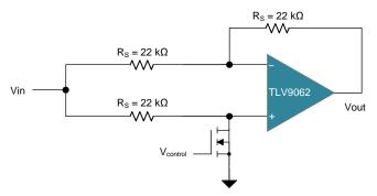
图 21. Polarity Reversal Circuit Explanation
