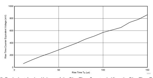
$\boxtimes$  47. Equivalent Analog Voltage of the Rise Time Counter (mV) vs the Rise Time T<sub>R</sub> ( $\mu$ s)
