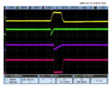
图 58. Pacemaker Detection Output (Rise Time T<sub>R</sub>) for 8-mV, 200-µs Pace Pulse
