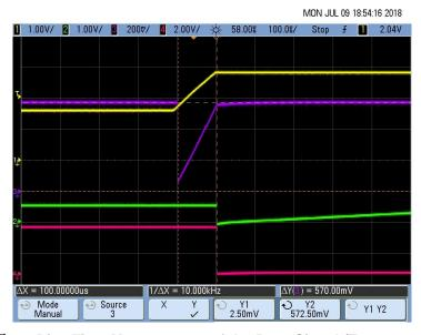
$\boxtimes$  43. Rise Time Measurement of the Pace Signal (T<sub>R</sub> = 100  $\mu$ s)
