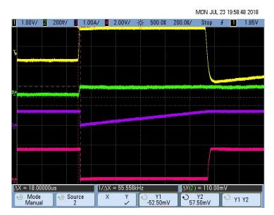
图 74. Pacemaker Detection Output (Rise Time T<sub>R</sub>) for 50-mV, 1-ms Pace Pulse
