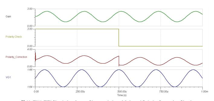
图 23. TINA-TI™ Simulation Output Characteristics of Gain and Polarity Correction Circuit
