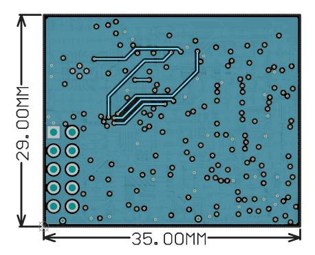
图 86. Power Plane of the Reference Design Board
