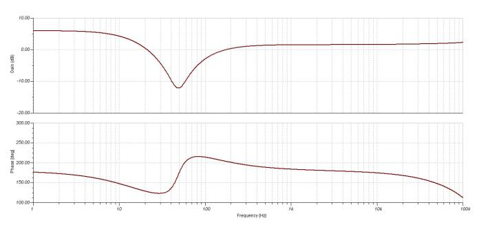
图 19. Frequency and Phase Response of the 50-Hz Notch Filter From 1 Hz to 100 kHz
