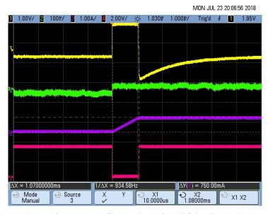
图 77. Pacemaker Detection Output (Pulse Duration T<sub>D</sub>) for 500-mV, 1-ms Pace Pulse
