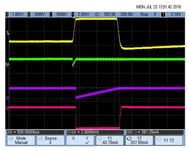
图 69. Pacemaker Detection Output (Pulse Duration T<sub>D</sub>) for 16-mV, 500-µs Pace Pulse
