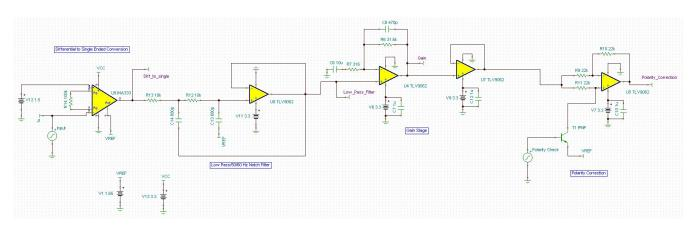
图 24. TINA-TI™ Schematic of the Entire Signal Processing Section
