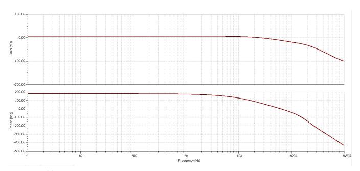
图 14. Frequency and Phase Response of the High-Pass Filter From 1 Hz to 1 MHz
