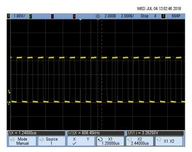
图 54. Clock (CLK B) Input to the Pulse Duration Counter
