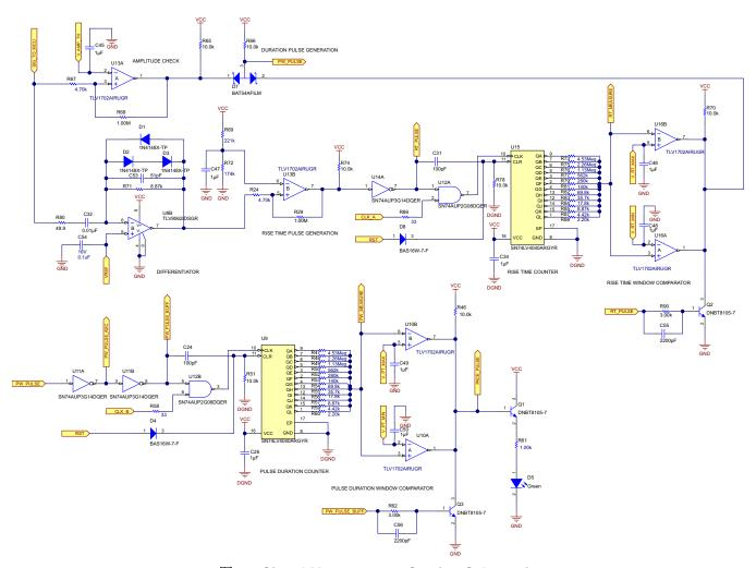
图 27. Signal Measurement Section Schematic
