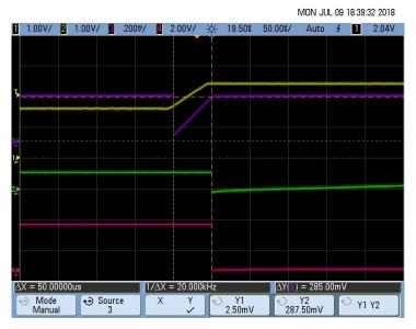
$\boxtimes$  44. Rise Time Measurement of the Pace Signal (T<sub>R</sub> = 50  $\mu$ s)
