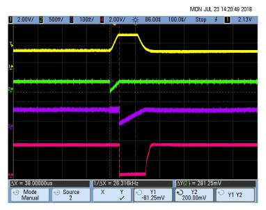
图 64. Pacemaker Detection Output (Rise Time T<sub>R</sub>) for 16-mV, 100-µs Pace Pulse
