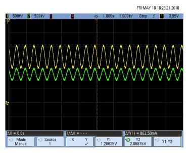
图 36. Output Characteristics of Differential to Single-Ended Converter (INA317)
