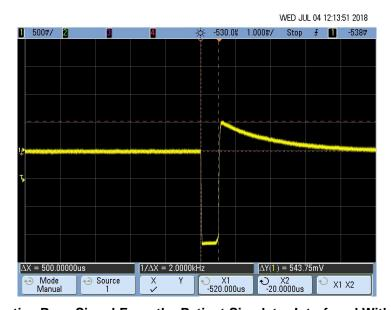
图 41. Negative Pace Signal From the Patient Simulator Interfaced With ADS1292
