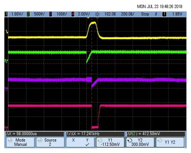
图 56. Pacemaker Detection Output (Rise Time T<sub>R</sub>) for 8-mV, 100-µs Pace Pulse
