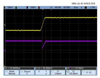
$\boxtimes$  45. Rise Time Measurement of the Pace Signal (T  $_{R}$  = 20  $\mu s)$
