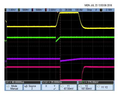
图 66. Pacemaker Detection Output (Rise Time T<sub>R</sub>) for 16-mV, 200-µs Pace Pulse
