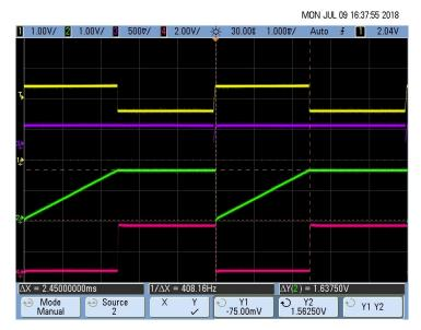
$\boxtimes$  51. Pulse Duration Measurement of the Pace Pulse (T<sub>D</sub> = 2.5 ms)
