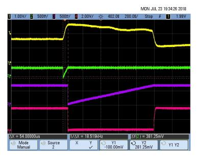
图 62. Pacemaker Detection Output (Rise Time T<sub>R</sub>) for 8-mV, 1-ms Pace Pulse
