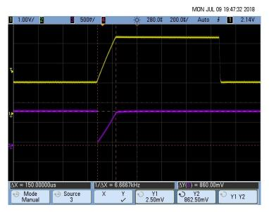
图 42. Rise Time Measurement of the Pace Signal ( $T_R$  = 150 μs)
