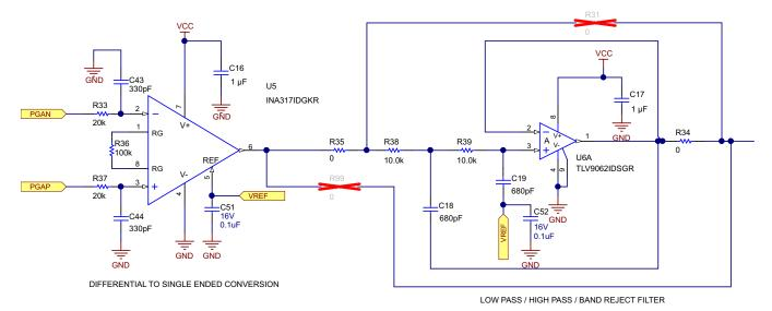
图 12. Low-Pass Filter Schematics for Filter Implementation
