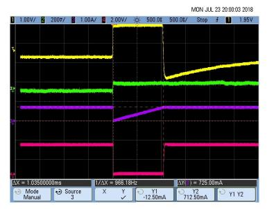
图 75. Pacemaker Detection Output (Pulse Duration T<sub>D</sub>) for 50-mV, 1-ms Pace Pulse
