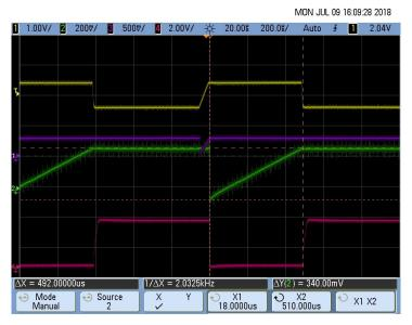
$\boxtimes$  48. Pulse Duration Measurement of the Pace Pulse (T<sub>D</sub> = 0.5 ms)
