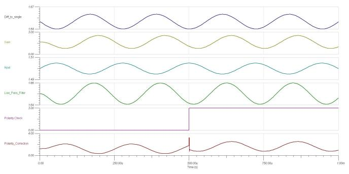
图 25. TINA-TI™ Simulation Output Characteristics of Entire Signal Processing Section
