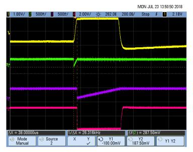
图 68. Pacemaker Detection Output (Rise Time T<sub>R</sub>) for 16-mV, 500-µs Pace Pulse
