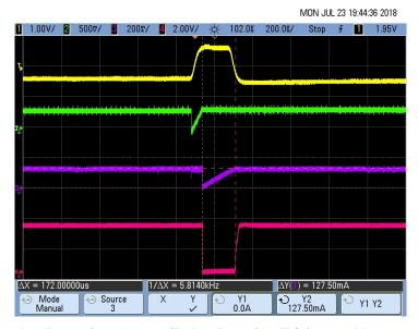
图 59. Pacemaker Detection Output (Pulse Duration T<sub>D</sub>) for 8-mV, 200-µs Pace Pulse
