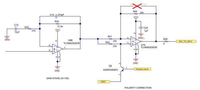
图 20. Gain and Polarity Correction Circuitry Schematic
