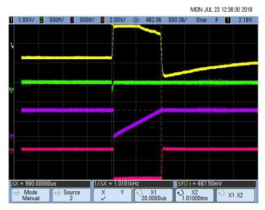
图 71. Pacemaker Detection Output (Pulse Duration T<sub>D</sub>) for 16-mV, 1-ms Pace Pulse
