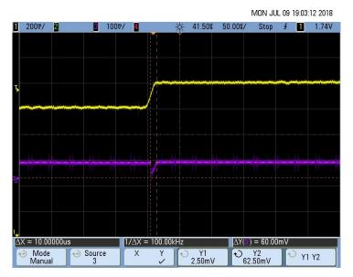
图 46. Rise Time Measurement of the Pace Signal ( $T_R = 10 \mu s$ )
