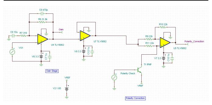
图 22. TINA-TI™ Simulation Schematic Gain and Polarity Correction Circuit
