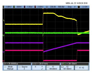
图 72. Pacemaker Detection Output (Rise Time T<sub>R</sub>) for 16 mV, 2 ms Pace Pulse
