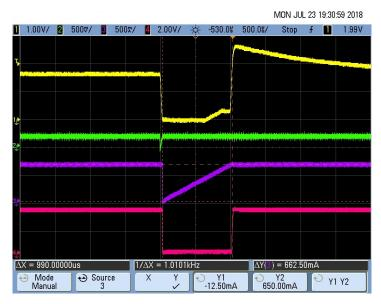
图 82. Negative Pace Signal Detection - Negative Pace Pulse Detected by setting the Polarity Check (CH-6) Output of the DAC Low`
