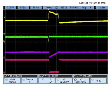
图 60. Pacemaker Detection Output (Rise Time T<sub>R</sub>) for 8-mV, 500-µs Pace Pulse
