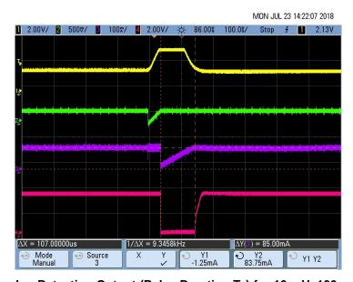
图 65. Pacemaker Detection Output (Pulse Duration T<sub>D</sub>) for 16-mV, 100-µs Pace Pulse
