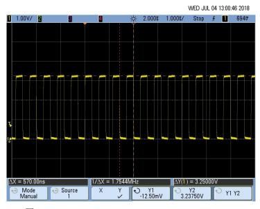
图 53. Clock (CLK A) Input to Rise Time Counter
