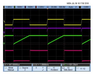
$\boxtimes$  49. Pulse Duration Measurement of the Pace Pulse (T<sub>D</sub> = 1 ms)
