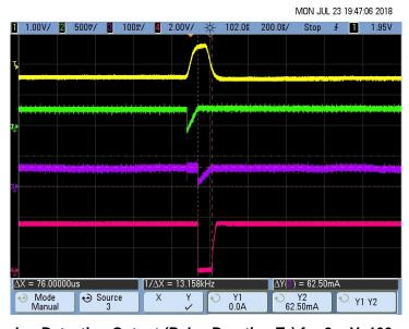
图 57. Pacemaker Detection Output (Pulse Duration T<sub>D</sub>) for 8-mV, 100-µs Pace Pulse
