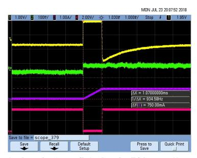
图 79. Pacemaker Detection Output (Pulse Duration T<sub>D</sub>) for 700-mV, 1-ms Pace Pulse
