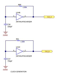
图 30. Circuitry Implemented to Generate Onboard Counter Clocks
