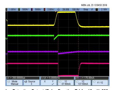
图 67. Pacemaker Detection Output (Pulse Duration T<sub>D</sub>) for 16-mV, 200-µs Pace Pulse
