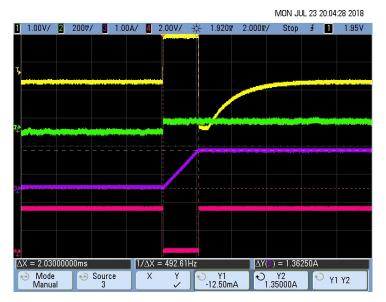
图 76. Pacemaker Detection Output (Pulse Duration T<sub>D</sub>) for 50-mV, 2-ms Pace Pulse
