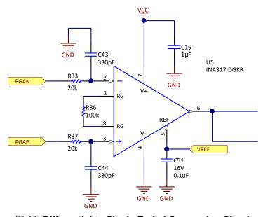
图 11. Differential to Single-Ended Conversion Circuit
