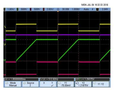
$\boxtimes$  50. Pulse Duration Measurement of the Pace Pulse (T<sub>D</sub> = 2 ms)
