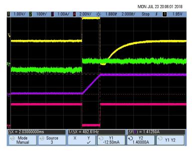
图 78. Pacemaker Detection Output (Pulse Duration T<sub>D</sub>) for 500-mV, 2-ms Pace Pulse
