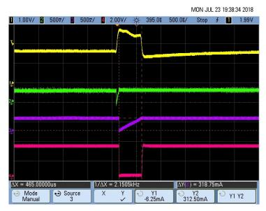
图 61. Pacemaker Detection Output (Pulse Duration T<sub>D</sub>) for 8-mV, 500-µs Pace Pulse
