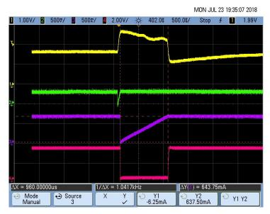
图 63. Pacemaker Detection Output (Pulse Duration T<sub>D</sub>) for 8-mV, 1-ms Pace Pulse
