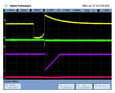
图 81. Negative Pace Signal Detection - Negative Pace Pulse Undetected
