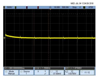
图 39. 16-mV Pace Signal 5 at the Output of the Gain Stage Interface With ADS1292
