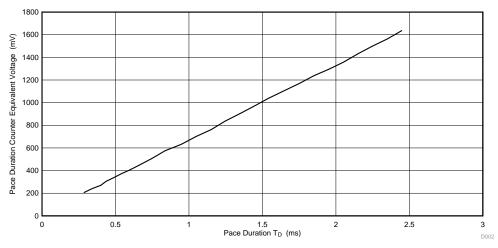
图 52. Equivalent Analog Voltage of the Pulse Duration Counter (mV) vs the Pulse Duration T<sub>D</sub> (ms)
