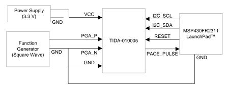
图 34. Test Setup to Evaluate the TIDA-010005 Using Function Generator
