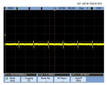
图 38. 5 mV ECG Signal at the Output of the Gain Stage Interfaced With ADS1292
