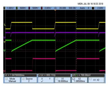
图 55. Pacemaker Detection Output for 8-mV, 100-µs Pace Pulse
