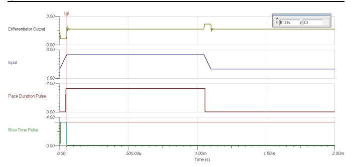
图 29. Simulation Output of the Signal Measurement Section Till TTL Pulse Generation
