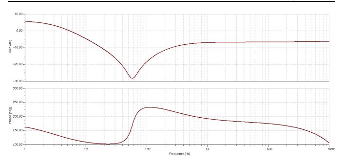
图 17. Frequency and Phase Response of the 60-Hz Notch Filter From 1 Hz to 100 kHz
