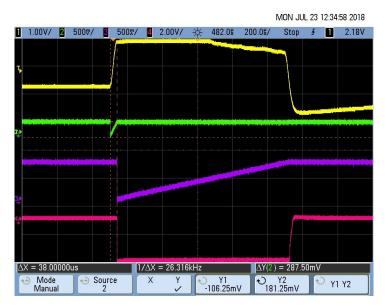
图 70. Pacemaker Detection Output (Rise Time T<sub>R</sub>) for 16-mV, 1-ms Pace Pulse
