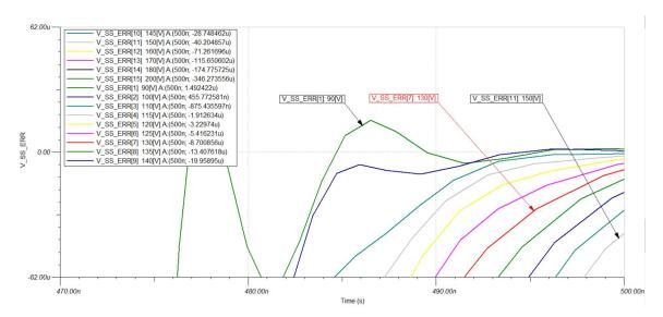
图 21. Parameter Stepping: Curves Settling Within ±0.5 LSB
