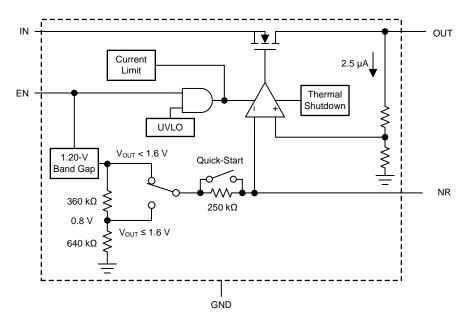
图 4. TPS717xx Functional Block Diagram
