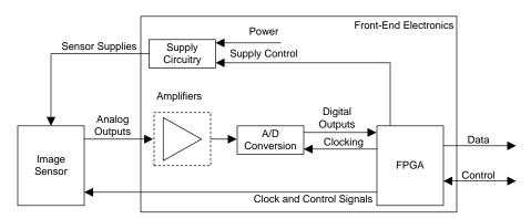
图 5. Basic Architecture of Camera Electronics
