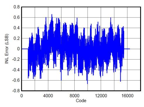
图 28. ADC INL Test With Driver Amplifier
