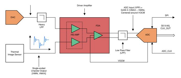
图 10. Conceptual Schematic of AFE Circuit for IR Imaging Applications
