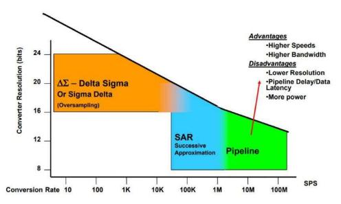
图 8. Converter Resolution Versus Conversion Rate
