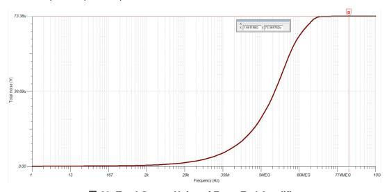
图 23. Total Output Noise of Front-End Amplifier
