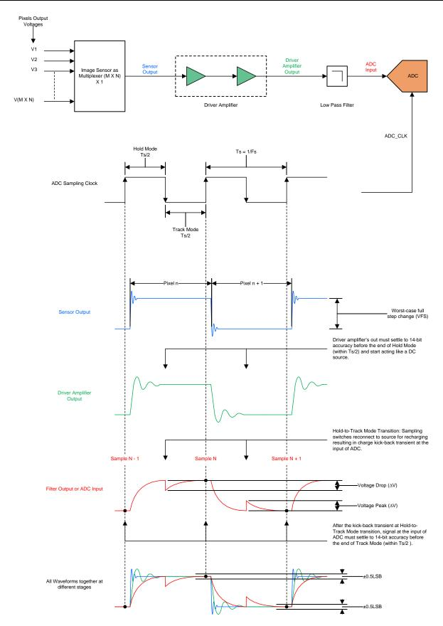
图 14. Waveforms at Different Stages in the Signal Chain
