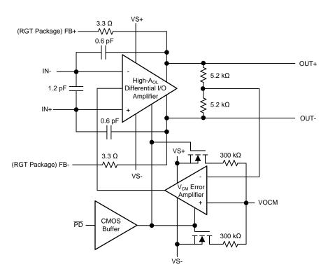
图 3. THS4551 Functional Block Diagram
