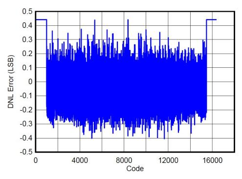
图 27. ADC DNL Test With Driver Amplifier
