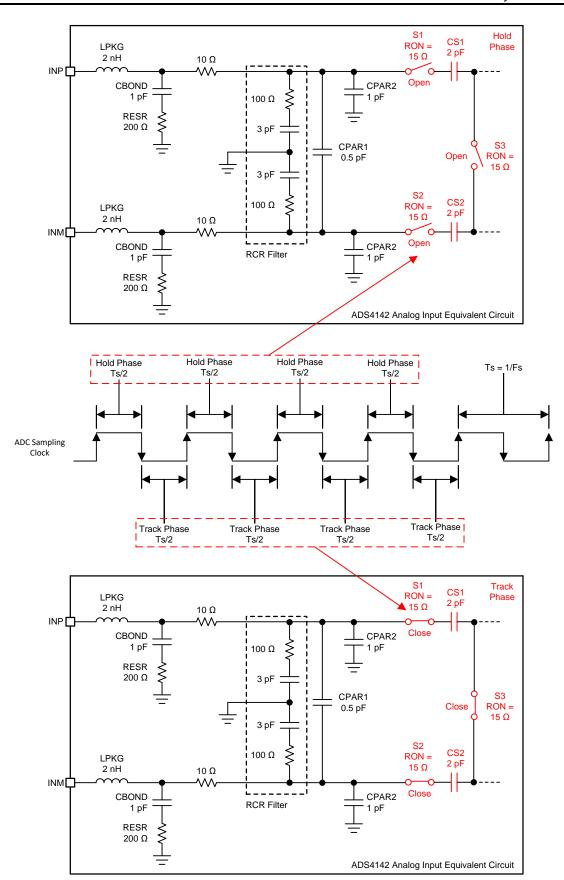
图 12. Sampling Switches S1 and S2
