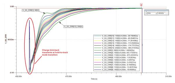
图 20. Parameter Stepping Simulation for Filter Resistors from 90  $\Omega$  to 200  $\Omega$
