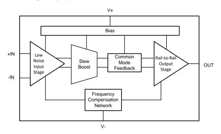
图 2. OPAx262 Functional Block Diagram
