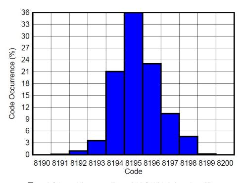
图 26. DC Input Histogram Test of ADC With Driver Amplifier
