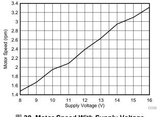
图 30. Motor Speed With Supply Voltage
