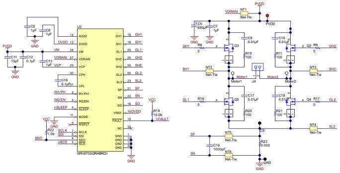
(1) The VM pin on the DRV88703-Q1 device supplies the PVDD voltage.
