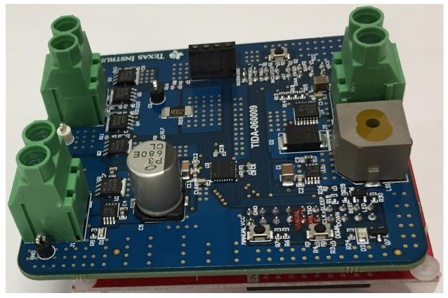
图 11. TIDA-060009 Connection With LaunchPad™ Development Kit
