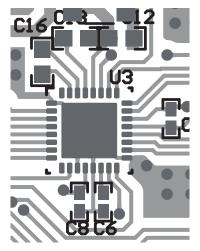
图 39. Bypass Capacitors of AVDD and DVDD
