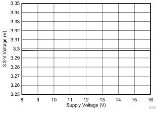
图 14. 3.3-V Voltage With Supply Voltage
