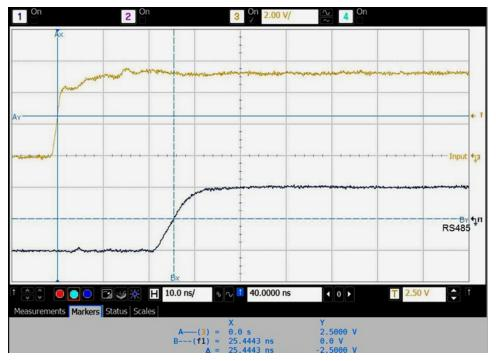
图 7. Propagation Delay (Low to High)
