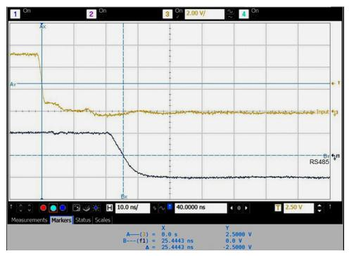
图 8. Propagation Delay (High to Low)
