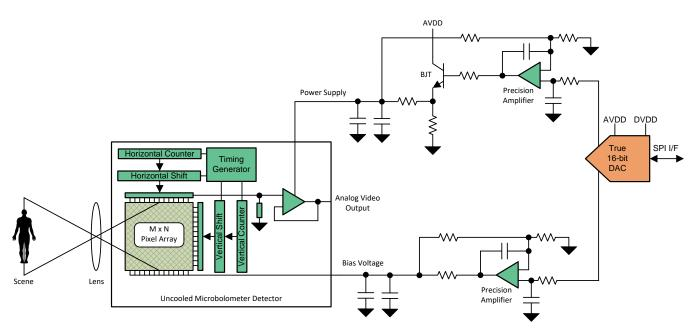
图 6. Bias Supply Generation Diagram
