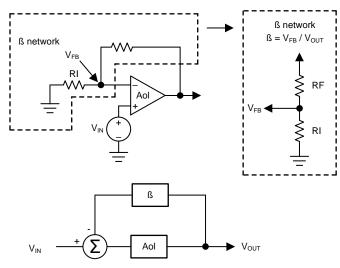
图 9. Model of Loop Gain for Op Amp
