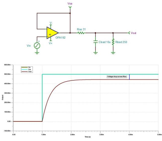
图 25. Riso Compensation Disadvantage
