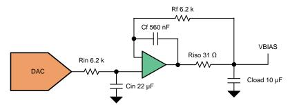
图 30. Proposed Ultra-Low Noise, Precision Bias Voltage Circuit
