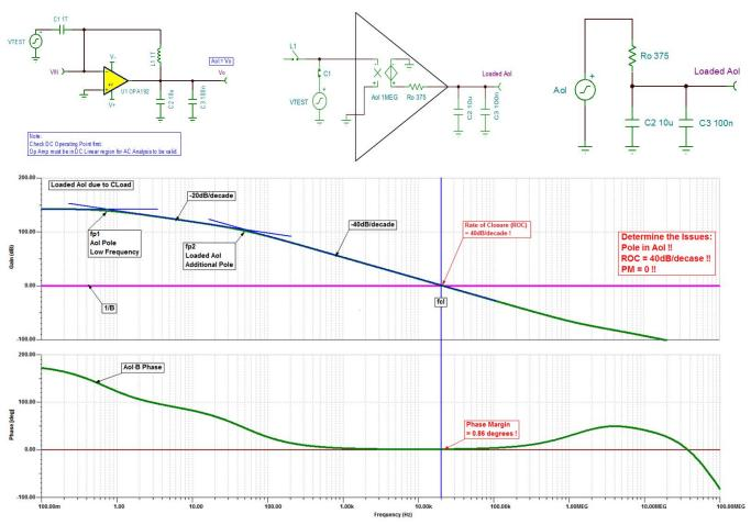
图 18. Bode Plot for OPA192 Unity-Gain Buffer With Capacitive Load
