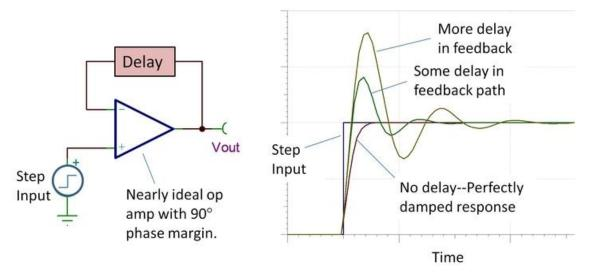
图 10. Effect of Delay in Feedback Loop on Stability of Op Amp
