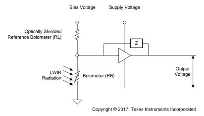
图 5. Simplified Diagram of Bolometer and Readout Circuit
