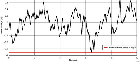
图 45. 0.1-Hz to 10-Hz Noise for Power Supply Circuit
