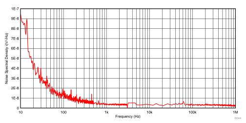
图 44. Spectral Voltage Noise Density for Bias Voltage Circuit
