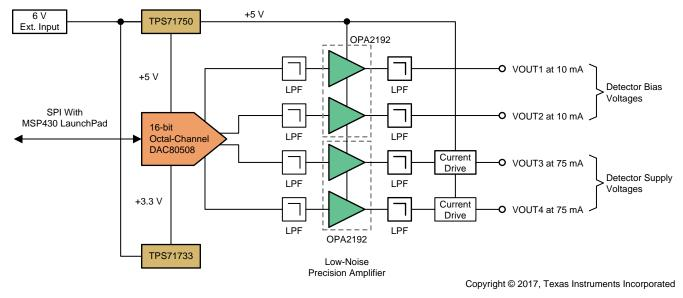
图 1. Block Diagram of TIDA-01583
