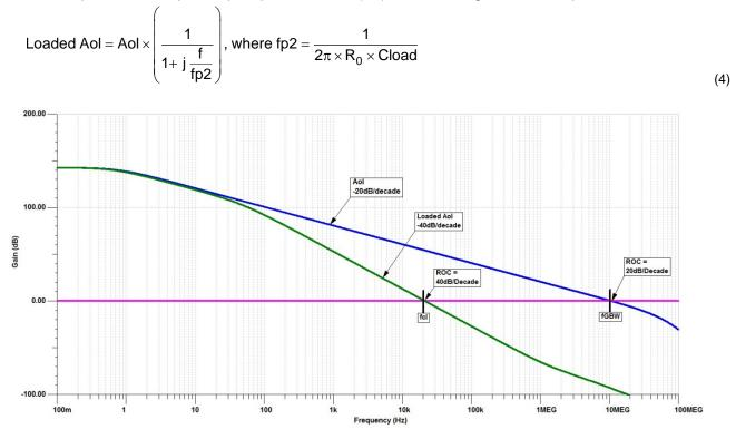
图 16. Bode Plot for OPA192 Unity-Gain Buffer With and Without Capacitive Load
