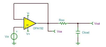
图 19. OPA192 Unity-Gain Buffer With Riso Stability Compensation
