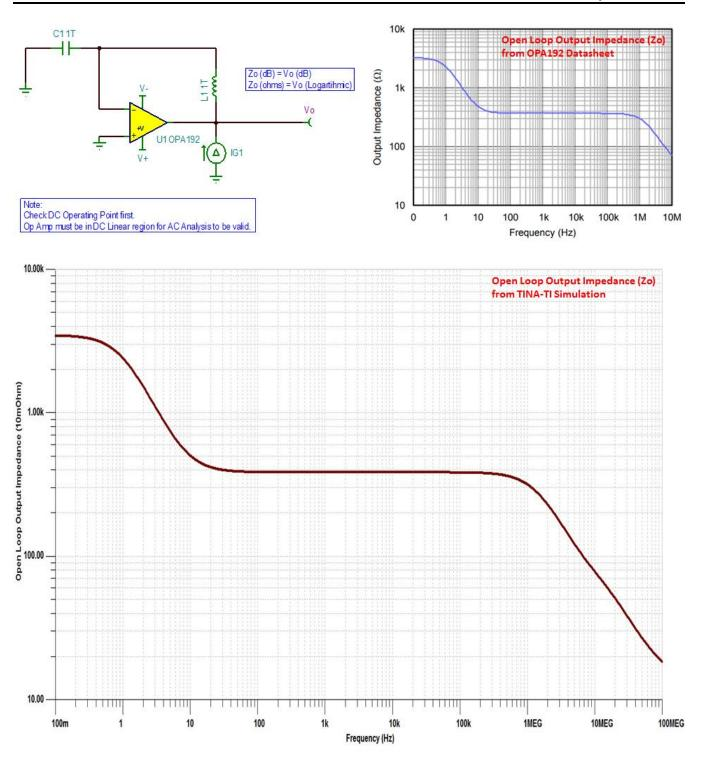
图 14. Open Loop Output Impedance (Zo) Test of OPA192 SPICE Macro Model
