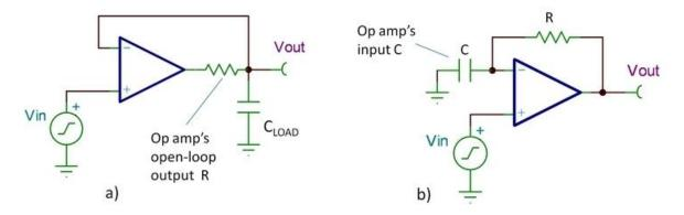
图 11. Sources of Delay in Feedback Path
