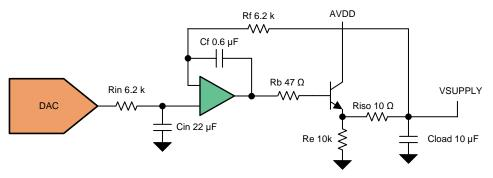
图 34. Final Proposed Circuit for Ultra-Low Noise, Precision Power Supply
