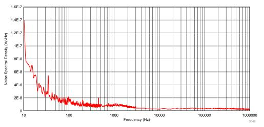
图 46. Noise Density of Spectral Voltage for Power Supply Circuit
