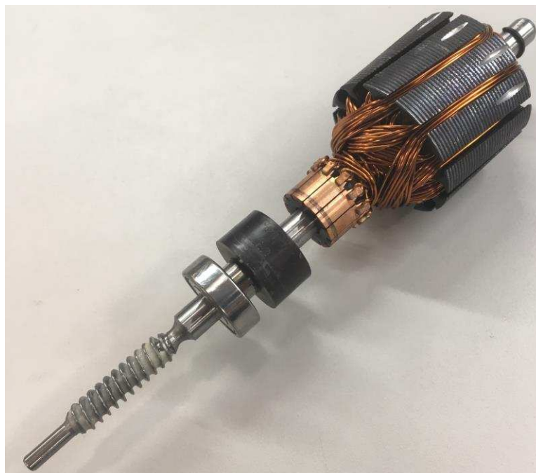
图 34. Detail of Typical Single-Speed Wiper Motor With Exposed Windings
