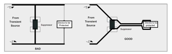
图 3. Interconnection of Transient Voltage Suppressor on PCB Diagram
