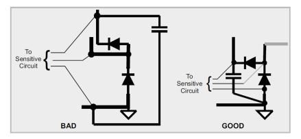
图 2. Interconnection to Clamping Devices
