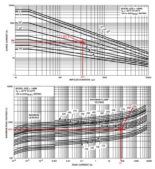
图 6. Using MOV Repetitive Surge Capability and Maximum Clamping Voltage Curves
