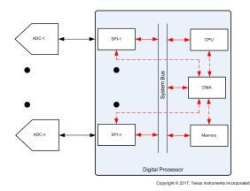
图 1. Interface Between Multiple ADCs With a Processor Using SPI
