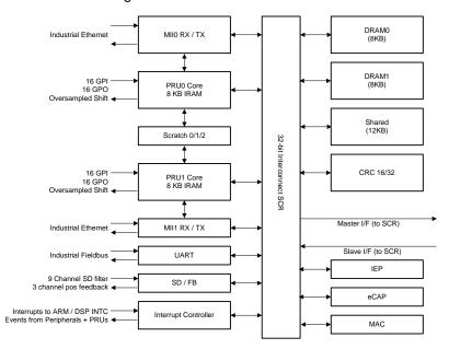
图 6. Functional Block Diagram of PRU-ICSS
