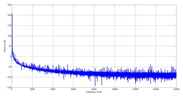
图 28. FFT Plot for AC Input Signal: Number of Points = 65536, f<sub>IN</sub> = 64 Hz, SFDR = 110 dB
