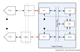
图 2. Data Acquisition System With Digital Isolation
