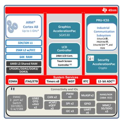
Figure 3. AM335x Block Diagram
