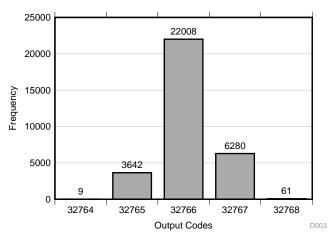
图 23. DC Histogram for One Channel: Sigma = 0.55, Code Peak = 32766
