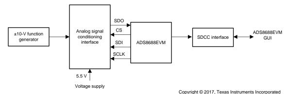
图 21. Test Setup for Functional Testing of Data Acquisition Board
