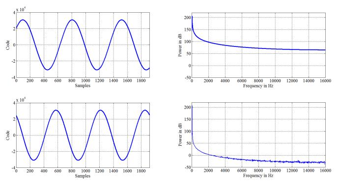
图 27. Comparison of AC Performance for Non-Coherent and Coherent Sampling
