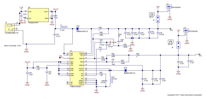
图 18. Schematic of Front-End DC/DC Converter Using TPS65131
