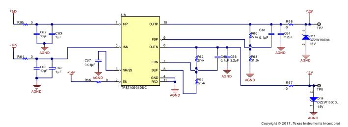
图 19. Schematic of Configuration for Dual-Channel LDO
