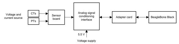
图 22. Test Setup for Performance Testing
