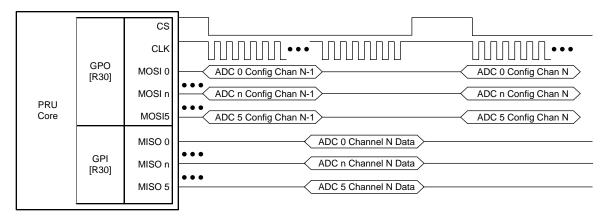
图 7. Interfacing Between ADC and PRU
