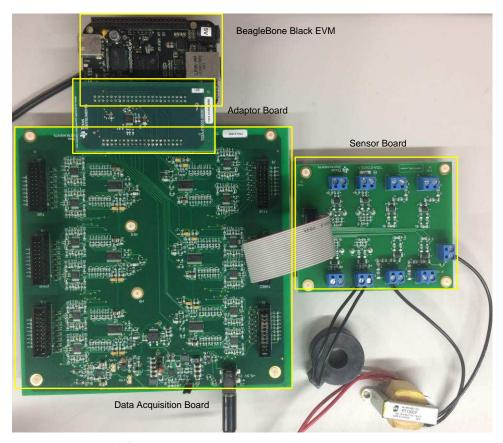
图 20. PCB Interconnection for TIDA-01555
