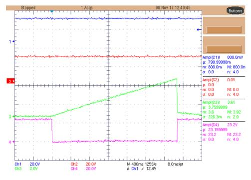
图 13. Short-Circuit Behavior—V<sub>in</sub> (1), GQ1 (2), C<sub>timer</sub> (3), V<sub>out</sub> (4)
