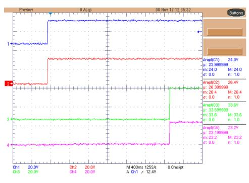
图 10. Power-up Sequence—V<sub>in</sub> (1), GQ1 (2), GQ2 (3), V<sub>out</sub> (4)
