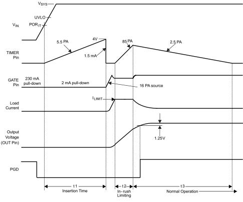
图 5. Power-up Sequence (Current Limit Only) of LM5069
