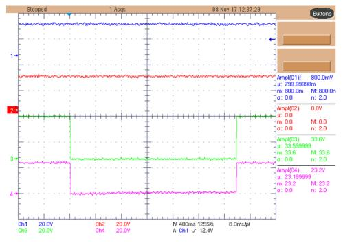
图 12. Short-Circuit Behavior—V<sub>in</sub> (1), GQ1 (2), GQ2 (3), V<sub>out</sub> (4)
