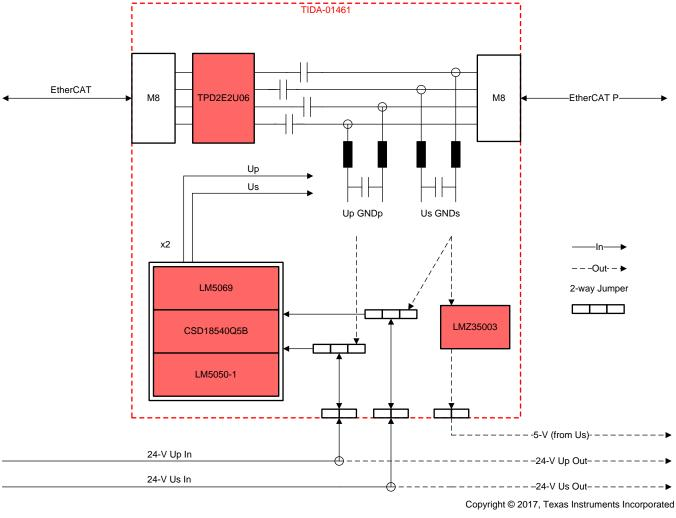
图 1. Block Diagram of TIDA-01461
