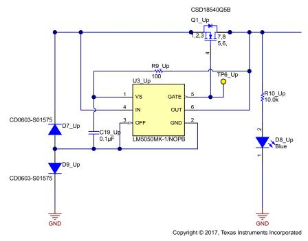
图 3. Schematic of Reverse Polarity Protection With LM5050-1
