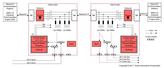
图 2. System Block Diagram With Two AMIC110 ICEs and Two TIDA-01461 Boards
