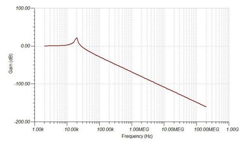
图 7. Bode Plot of Second-Order LC Low-Pass Filter (L = 6.8  $\mu$ H and C = 10  $\mu$ F)
