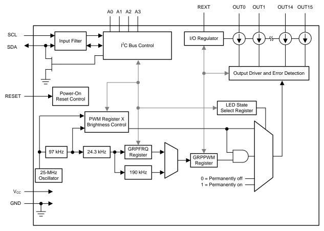
图 3. TLC59116-Q1 Block Diagram—OUT0 to OUT15 as Constant Current Sink Outputs
