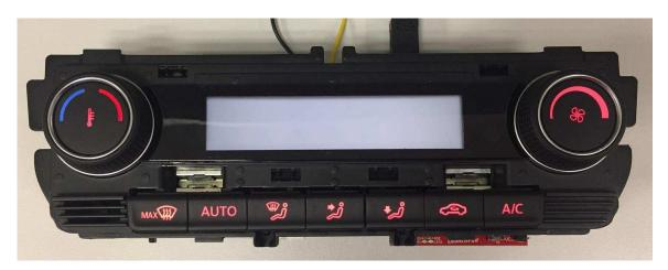
图 20. LED Dimming With 45% Duty Cycle
