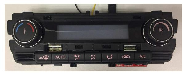
图 18. LED Dimming With 4% Duty Cycle
