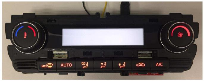
图 13. TIDA-01500 into HMI Housing
