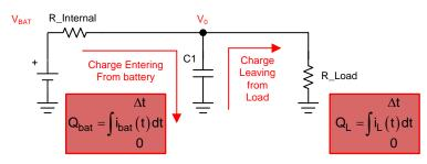
图 5. Battery Power Schematic
