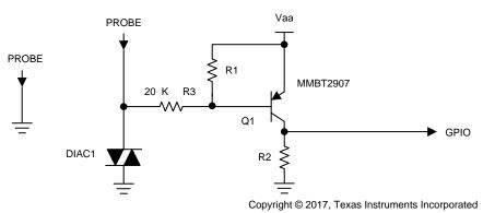
图 7. TIDA-01519 Leak Detection Schematic
