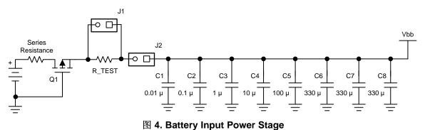
The power source for this reference design is an Energizer® CR2032 lithium-ion coin cell. This battery is chosen for its low cost and high capacity-to-size ratio. The voltage characteristics of a lithium-ion CR2032 coin cell battery are also ideal. The output voltage remains relatively flat throughout the discharge life until the cell is nearly depleted. When the cell is depleted, the output voltage drops off relatively quickly.
