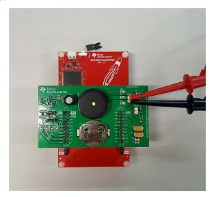
图 25. Test Setup of Main Supply Current Consumption
