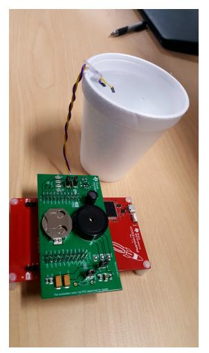
图 23. Test Setup of Water Leak Detection
