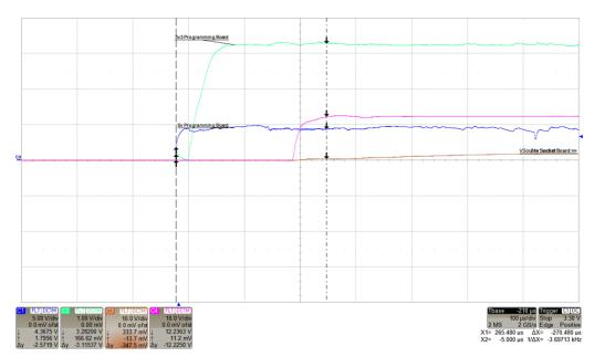
图 17. VSource Socket Board Start-up Time: 270 µs
