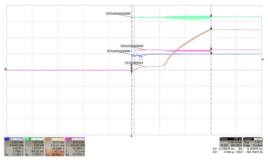
图 18. 24-V Socket Board Startup Time: 6.24 ms
