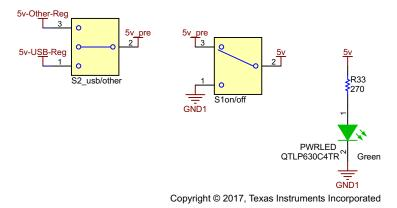
图 4. TIDA-01373 System Control Switches—Programming Board
