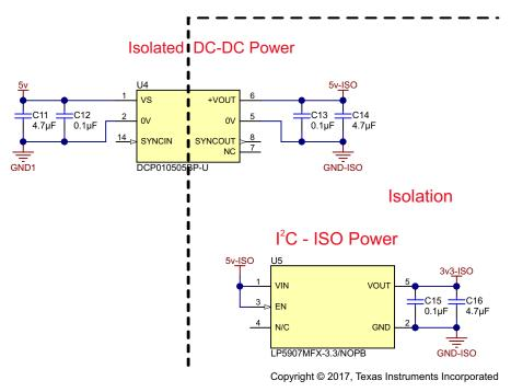
图 10. Power Isolation Circuitry—Programming Board
