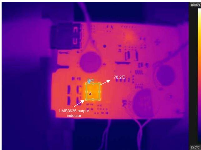
图 43. LMS3635-Q1 Output Inductor at 78.2°C:
