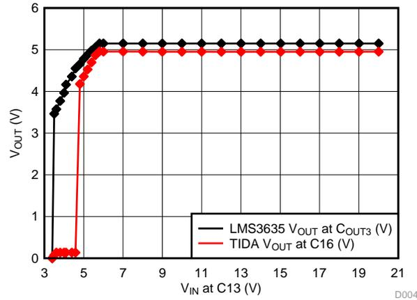
图 36.  $V_{IN} = 0\text{ V}$  to  $20\text{ V}$  Measured at C13,  $1.7\text{-}\Omega$  Load
