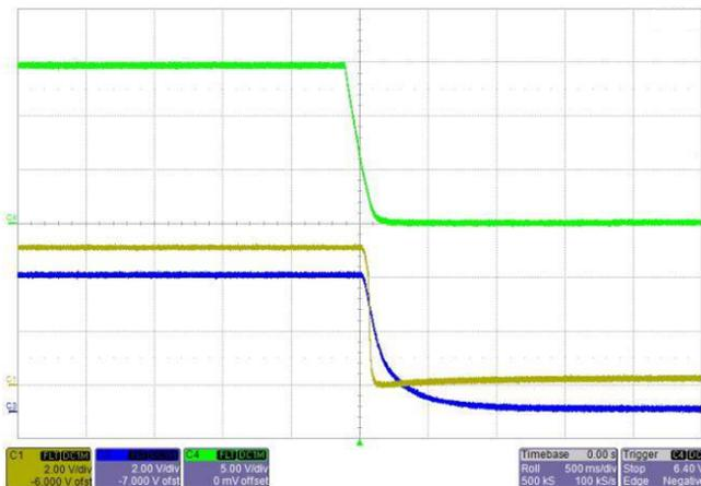
图 28.  $V_{IN} = 14.5$  V (Green), LMS3635 5  $V_{OUT}$  (Blue), USB 5 V (Yellow)—Shutdown = 150 ms at  $I_{OUT} = 0$  A
