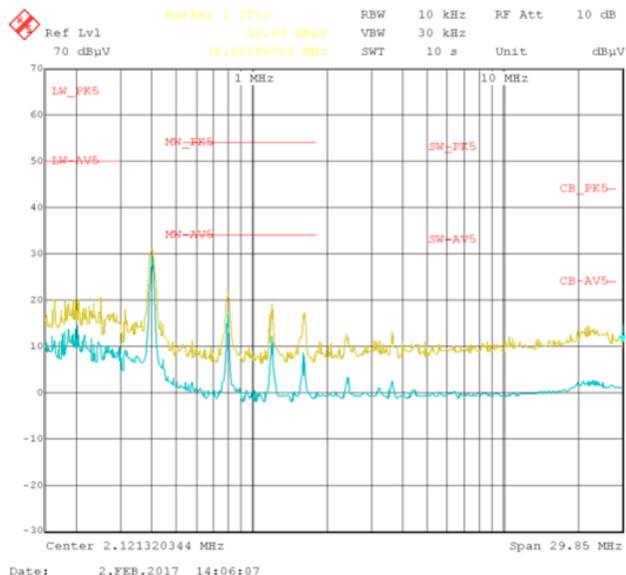
图 58. Low-Frequency Testing (100 kHz to 30 MHz) of Conducted EMI Performance
