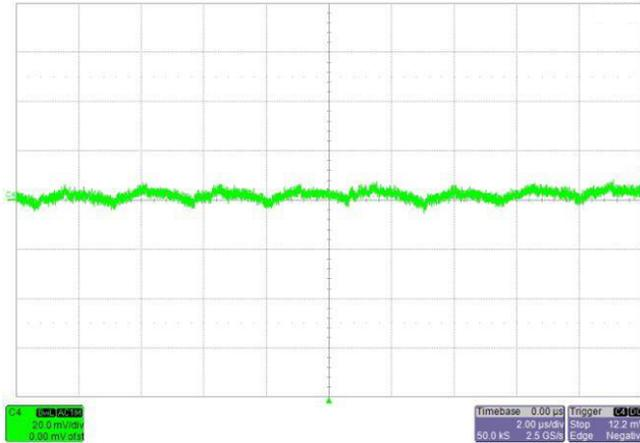
图 39.  $V_{IN} = 14.5\text{-V}$  Output Ripple Measured at COUT3 With No Load
