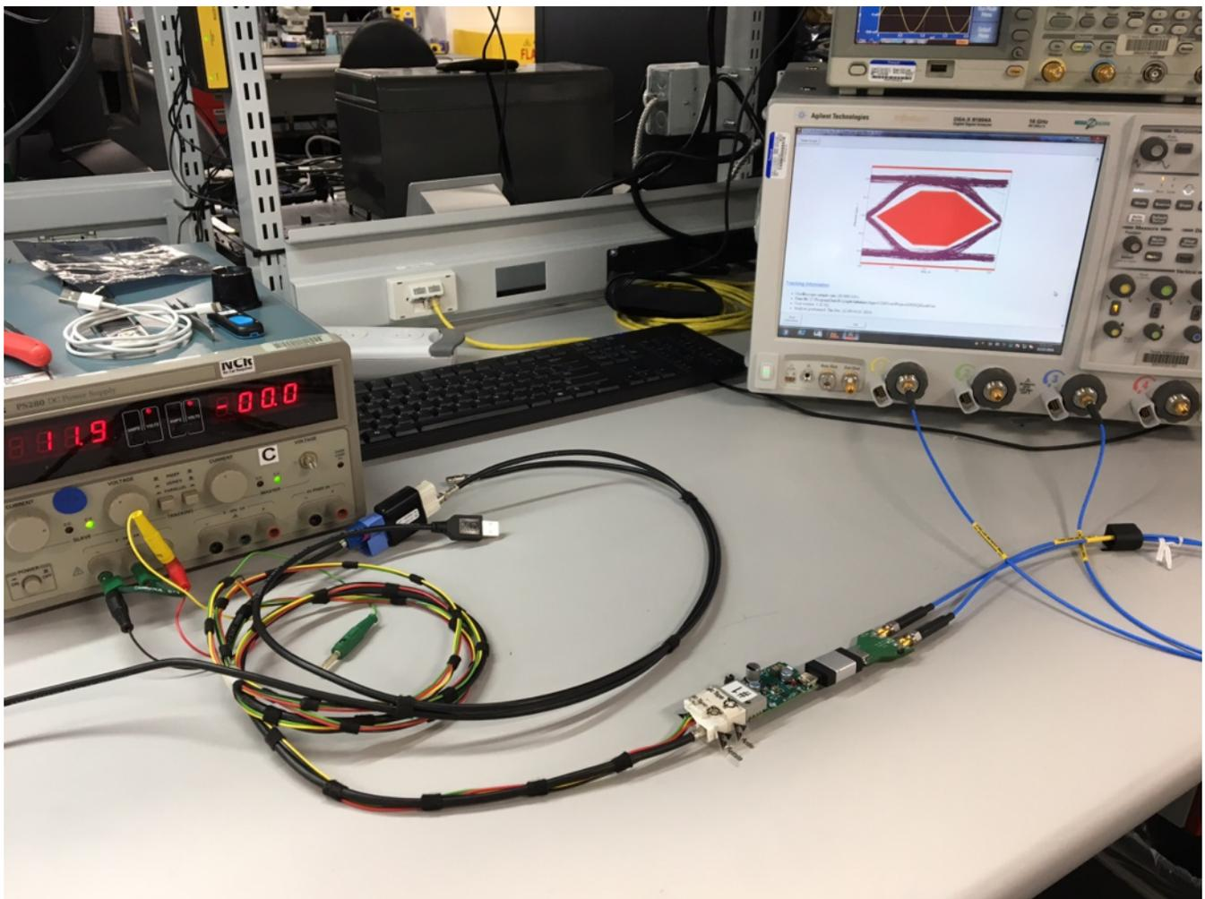
图 48. Near-End Test Setup Photo
