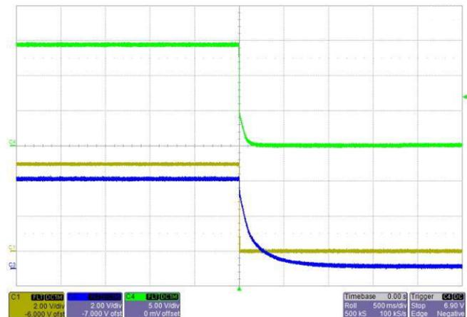
图 29.  $V_{IN} = 14.5$  V (Green), LMS3635 5  $V_{OUT}$  (Blue), USB 5 V (Yellow)—Shutdown = 50 ms at  $I_{OUT} = 3$  A
