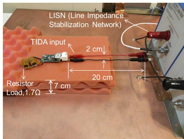
图 55. TIDA-01432 CISPR 25 Class 5 Testing
