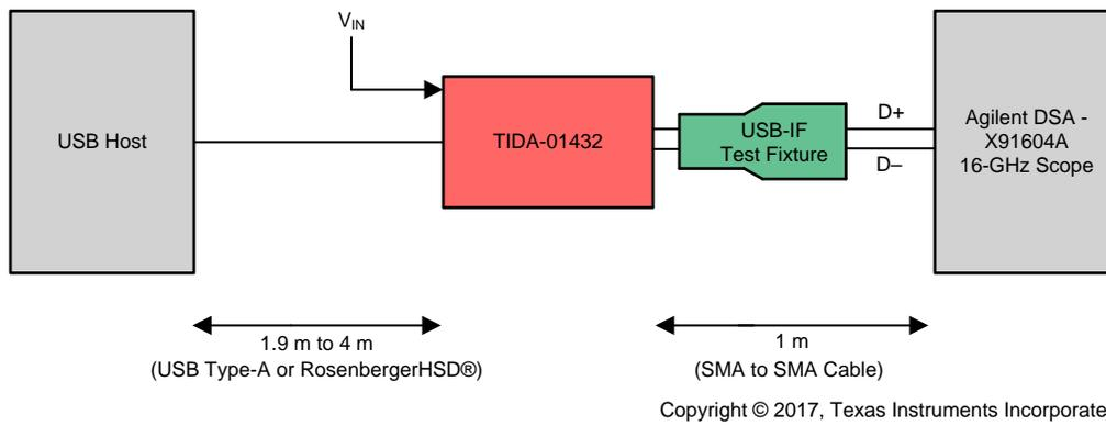
图 47. Block Diagram of Near-End Test Setup
