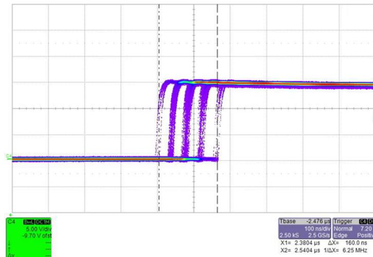
图 32. Spread Spectrum is  $\pm 3\%$  of Switching Frequency
