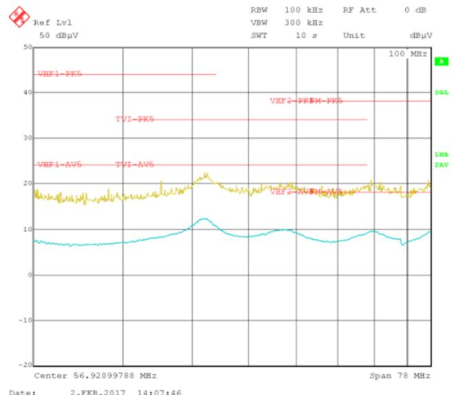
图 59. High-Frequency Testing (30 MHz to 100 MHz) of Conducted EMI Performance
