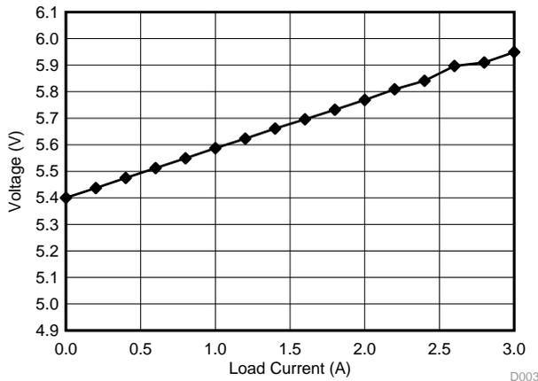
show the differences between load regulation of the board when cable compensation is enabled and disabled.
