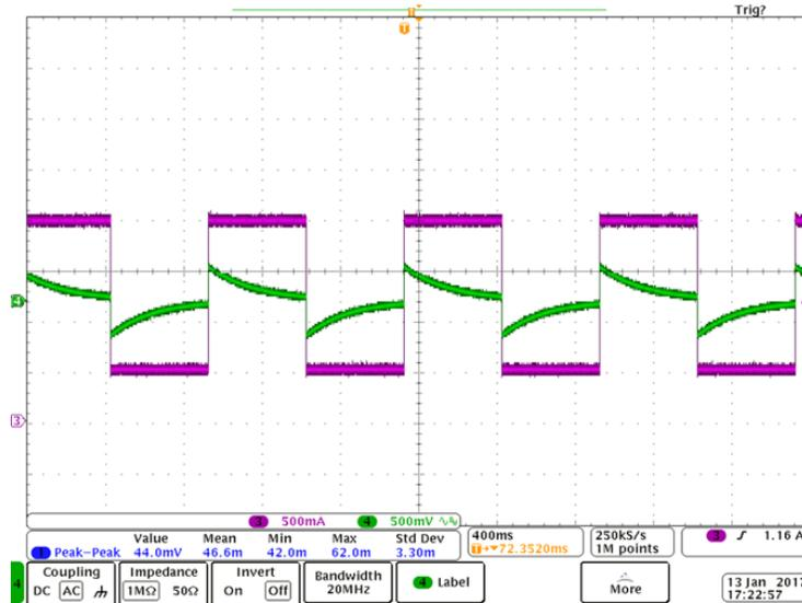
图 33.  $V_{IN} = 13.5\text{ V}$ , Load Step = 0.5 A to 2 A (Switching), Load Transient = 250 mV at LMS3635  $V_{OUT}$  (COUT3)
