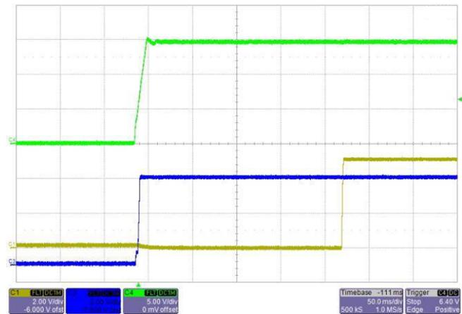
图 27.  $V_{IN} = 14.5$  V (Green), LMS3635 5  $V_{OUT}$  (Blue), USB 5 V (Yellow)—Start-Up = 10 ms at  $I_{OUT} = 3$  A
