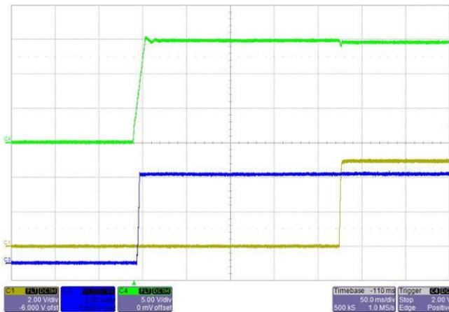
图 26.  $V_{IN} = 14.5$  V (Green), LMS3635 5  $V_{OUT}$  (Blue), USB 5 V (Yellow)—Start-Up = 15 ms at  $I_{OUT} = 0$  A
