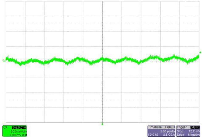
图 40.  $V_{IN} = 14.5\text{-V}$  Output Ripple Measured at COUT3 With 3-A Load
