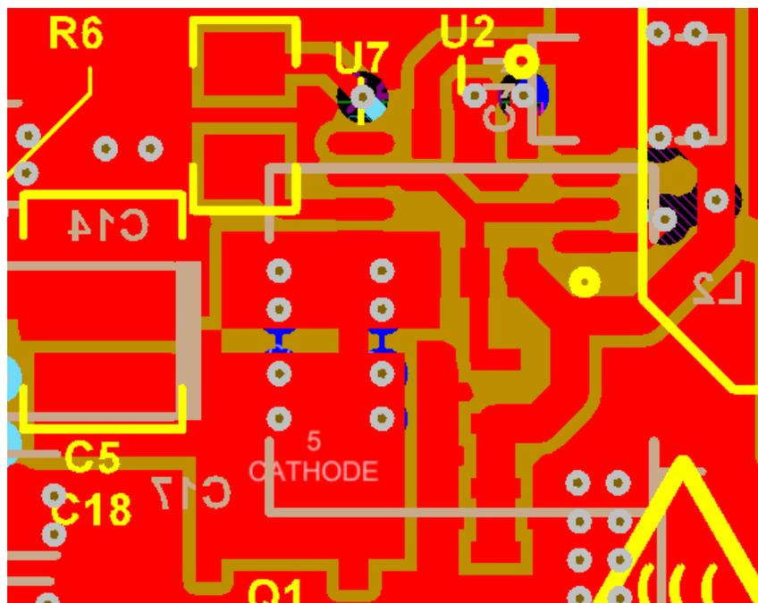
图 20. Reverse Battery Protection Layout
