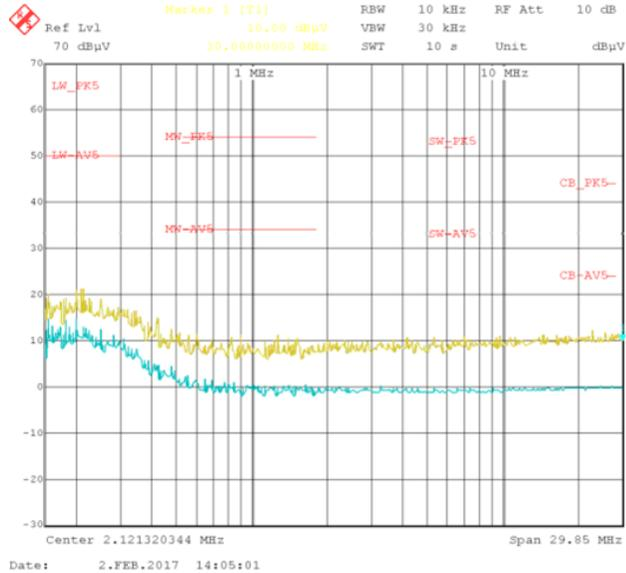
图 56. Low-Frequency Testing (100 kHz to 30 MHz) of Conducted EMI Performance
