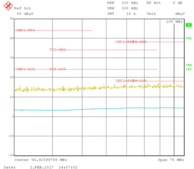
图 57. High-Frequency Testing (30 MHz to 100 MHz) of Conducted EMI Performance
