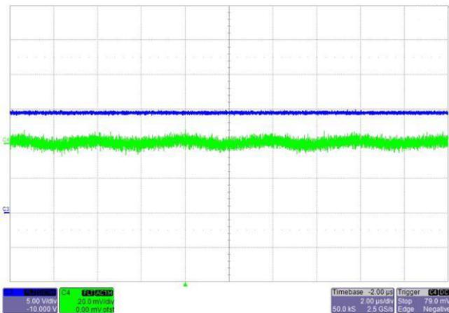
图 37.  $V_{IN} = 14.5\text{ V}$  Measured at C13 With No Load
