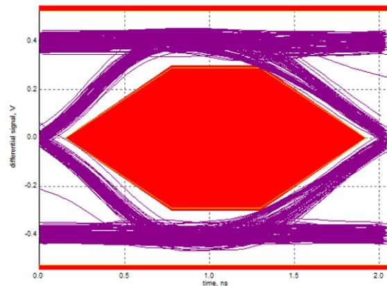
图 50. Near-End USB-IF Test With TUSB213-Q1 Enabled
