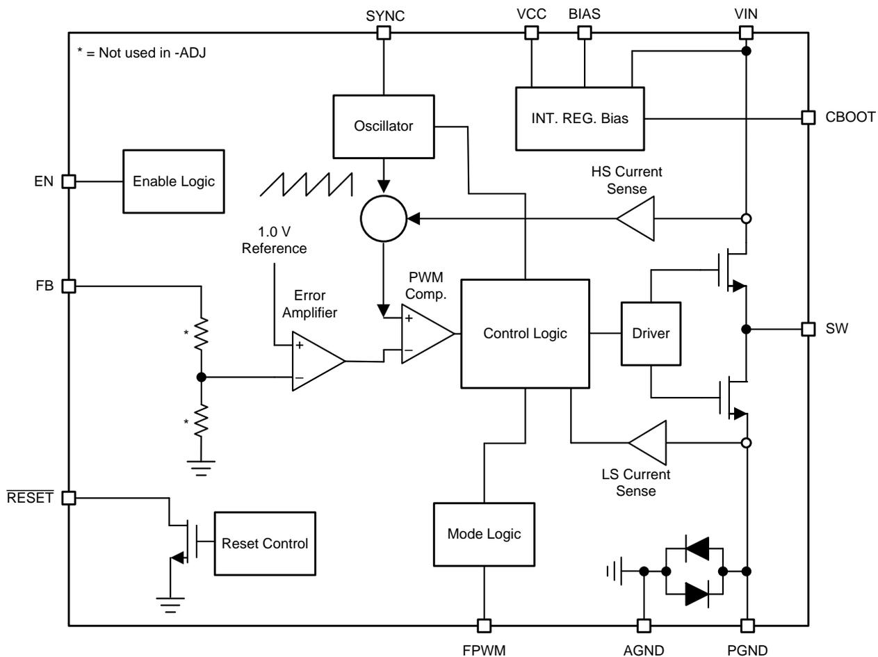
图 6. LMS3635-Q1 Functional Block Diagram
