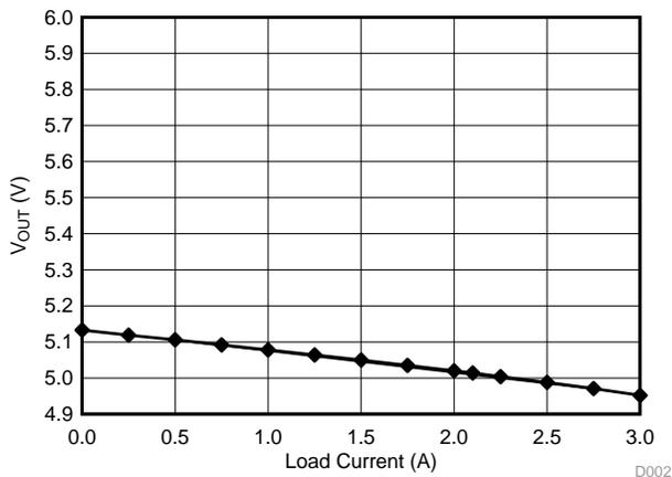
图 34.  $V_{IN} = 14.5$  Measured at C13, USB  $V_{OUT}$  Measured at C16, Cable Compensation Disabled
