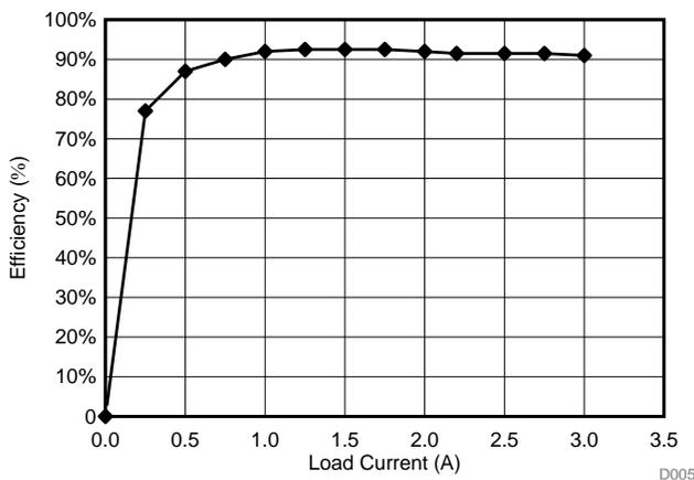
图 41.  $V_{IN} = 14.5\text{ V}$  Measured at C13 With TIDA-01432 Efficiency—Measured at COUT3
