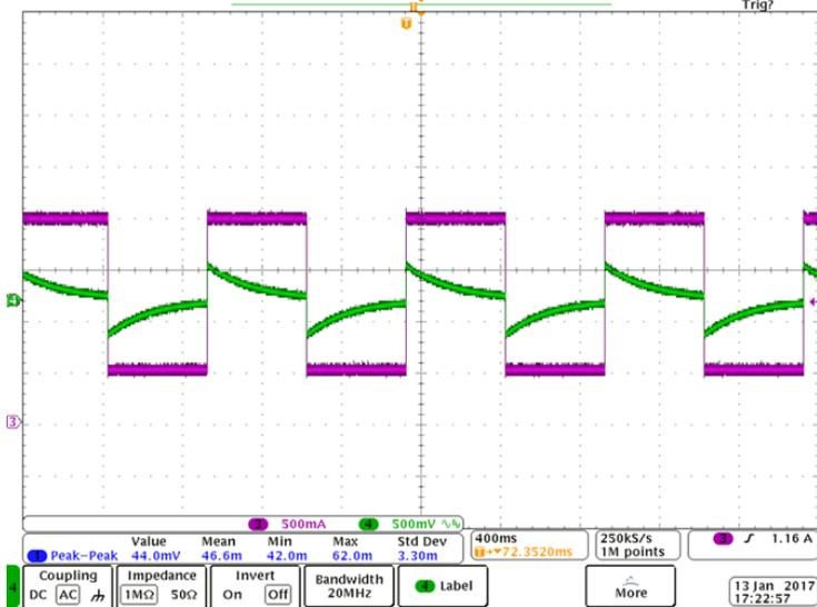
shows the load current versus the output voltage measurement (AC coupled).
