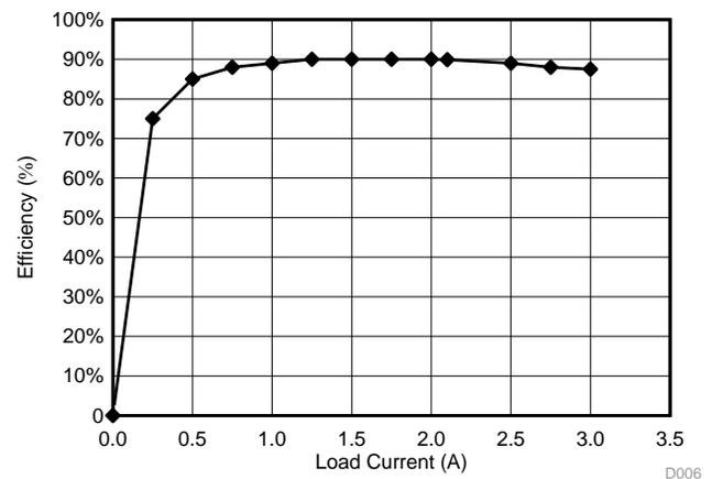
图 42.  $V_{IN} = 14.5\text{ V}$  Measured at C16 and LMS3635-Q1—Measured at COUT3
