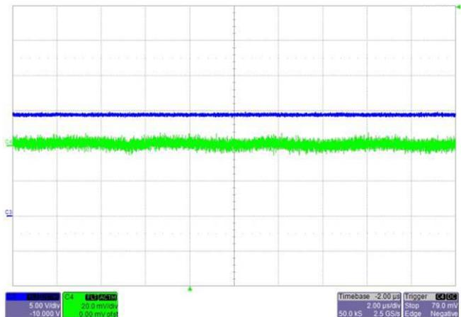
图 38.  $V_{IN} = 14.5\text{ V}$  Measured at C13 With 3-A Load
