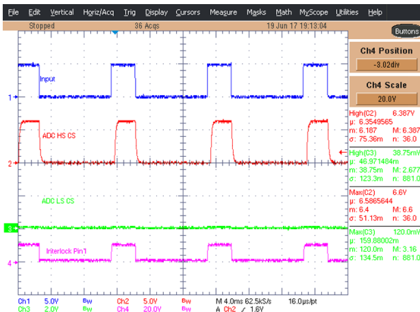
图 45. TIDA-01445 Short Circuit to Ground at Pin 2
