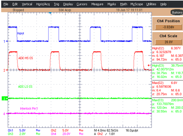
图 44. TIDA-01445 Short Circuit to Ground at Pin 1
