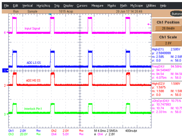
图 38. TIDA-01445 for 95 Hz and 10% Duty Cycle
