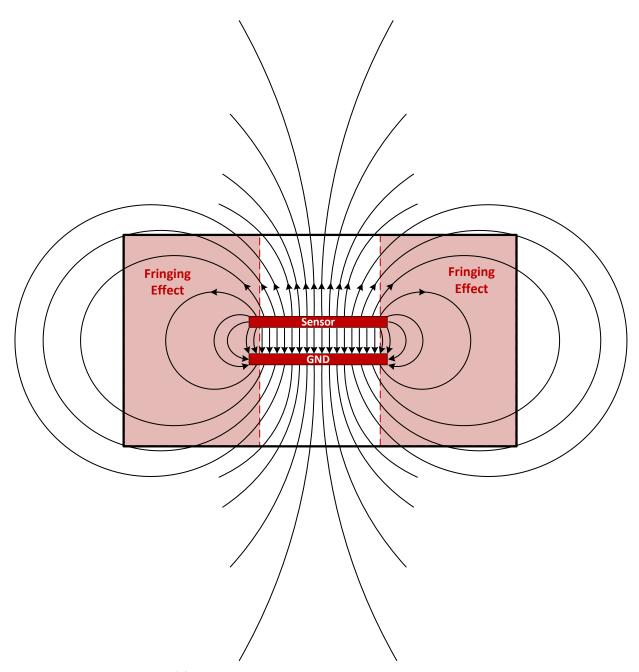
图 6. Electric Fields of Parallel Plate Capacitor
