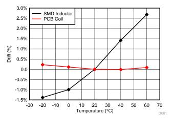
图 32. Capacitance Temperature Drift For PCB Coil and Common SMD Inductor
