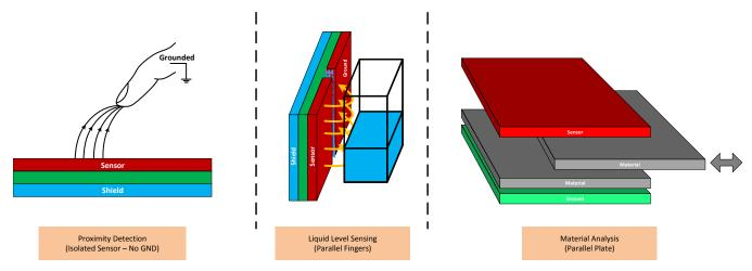
图 7. Basic Implements for Capacitive Sensing
