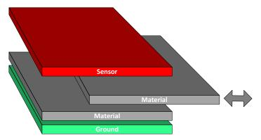
图 10. Parallel Plate Topology for Material Analysis
