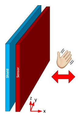
图 14. Single-Sensor Topology for Human Recognition
