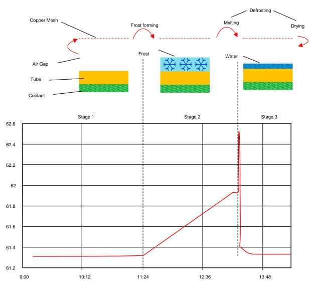
图 17. Capacitance Change in Single Cycle
