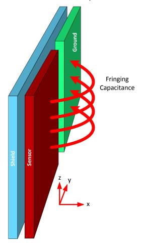
图 11. Parallel Fingers (GND Sensor) Topology
