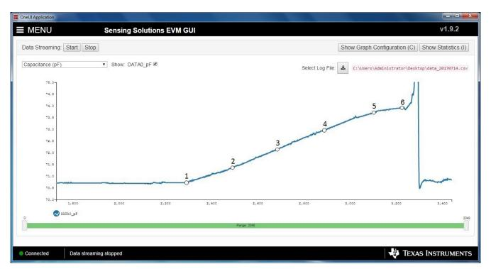
图 30. Sensed Capacitance During Frost Forming Process
