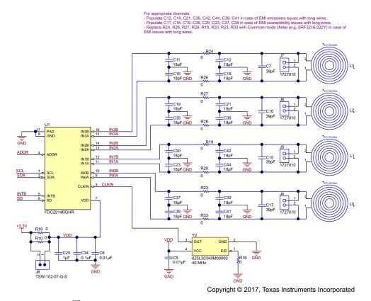
图 9. Schematic for Capacitance Detection Circuits
