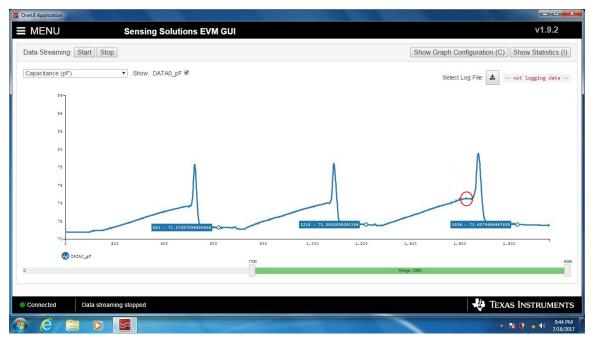
图 37. Capacitance Curve in Multi-Cycle Repeatability Test
