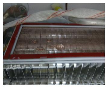
图 34. Waterdrop on Surface of Sensor
