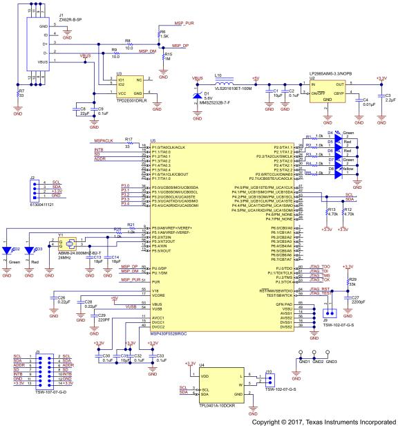
图 21. Schematic for Auxiliary Control Board
