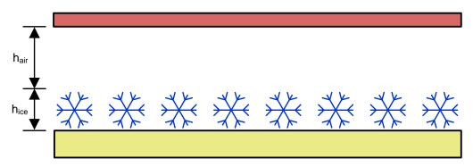
图 8. Model for Frost and Ice Detection Based on Capacitance
