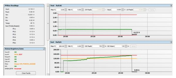
图 28. Overcurrent Shutdown as Seen in Fusion GUI
