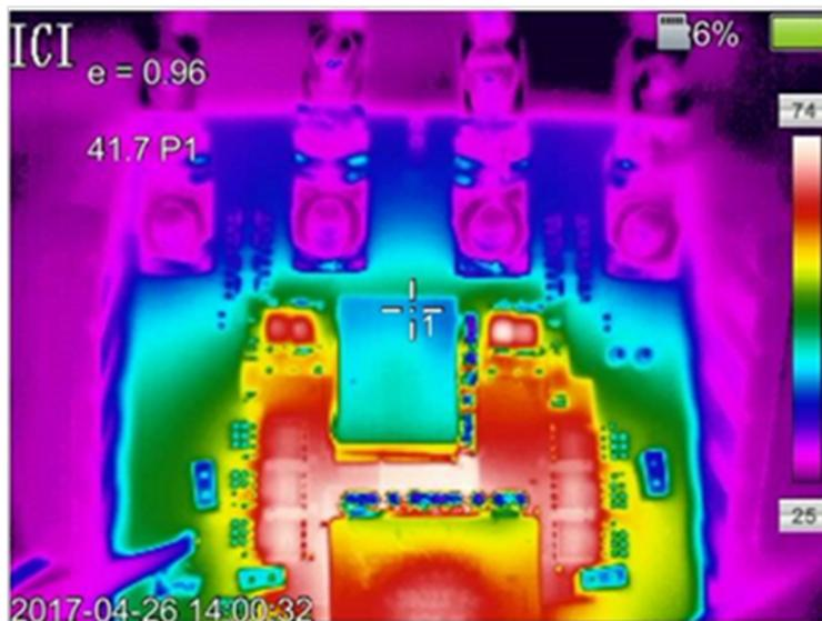
图 37. Thermal Image of Output Inductor (L1)
