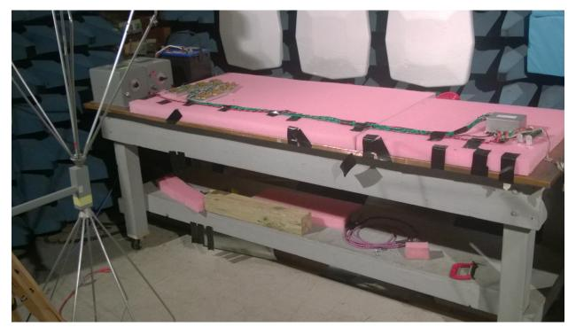
图 20. Radiated Emissions Test Setup
