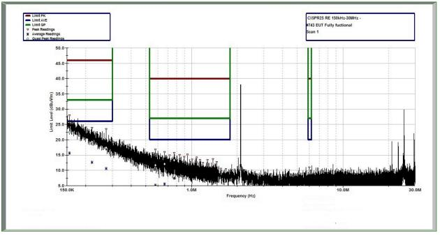
图 26. CISPR 25 Radiated Emissions: 150 kHz to 30 MHz
