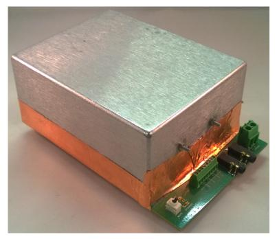
图 18. TIDA-00743 in Metal Box for EMI Tests
