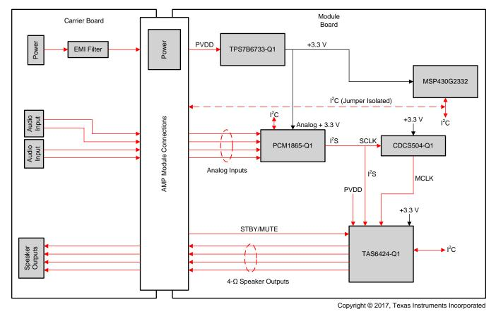
图 14. Block Diagram for Module Board and Carrier Board
