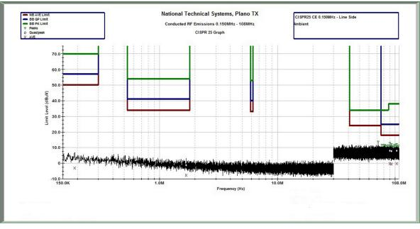
图 23. CISPR 25 Conducted Emissions Ambient Scan
