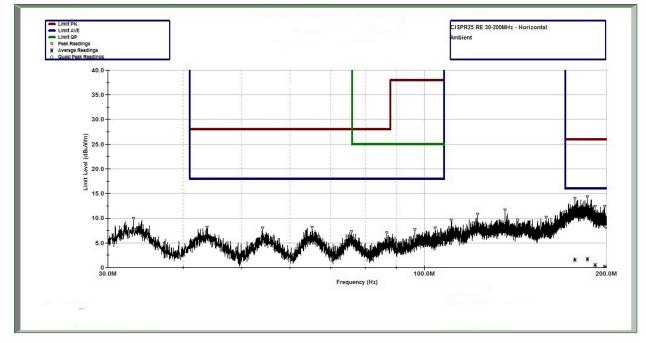
图 27. CISPR 25 Radiated Emissions: 30 MHz to 200 MHz, Horizontal Antenna Orientation, Ambient Scan
