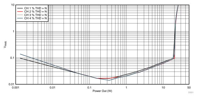
图 21. Power Output (W) versus THD + Noise (%)—Channels Driven Individually
