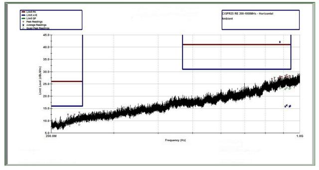
图 31. CISPR 25 Radiated Emissions: 200 MHz to 1 GHz, Horizontal Antenna Orientation, Ambient Scan
