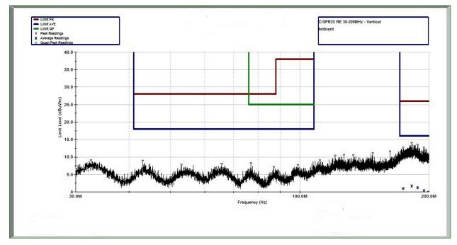
图 28. CISPR 25 Radiated Emissions: 30 MHz to 200 MHz, Vertical Antenna Orientation, Ambient Scan
