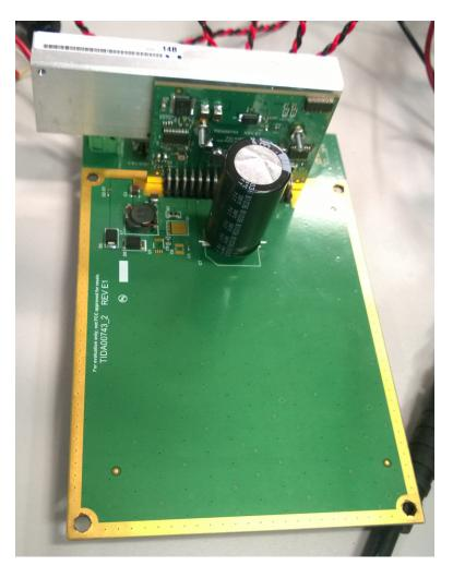
图 15. TIDA-00743 Module Board With Heat Sink Attached to Carrier Board
