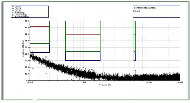
图 25. CISPR 25 Radiated Emissions: 150 kHz to 30 MHz, Ambient
