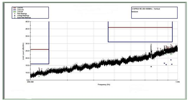
图 32. CISPR 25 Radiated Emissions: 200 MHz to 1 GHz, Vertical Antenna Orientation, Ambient Scan
