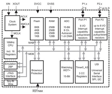
图 6. MSP430G2332 Functional Block Diagram
