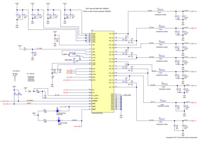
图 11. TAS6424-Q1 Class-D Power Audio Amplifier Circuit
